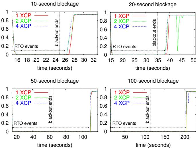
Fig. 13. XCP bandwidth utilization during and after blockage of various length
