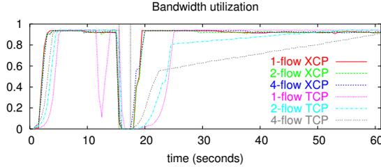
Fig. 12. XCP behavior around 2-second blockage (15th-17th second)
