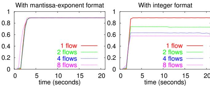
Fig. 3. Bandwidth utilization (total goodput of all flows as a ratio of raw bandwidth) comparison when 1, 2, 4, or 8 flows sharing the same bottleneck.
