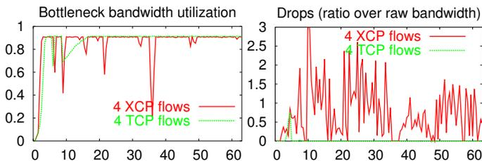
Fig. 17. XCP and TCP performance in the second experiment
