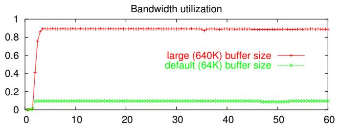
Fig. 8. XCP bandwidth utilization under different parameter tuning.
