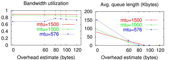
Fig. 7. Per-packet overhead estimates
