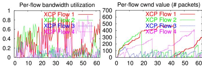
Fig. 16. XCP fails to converge (case 1)
