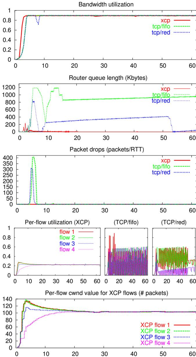
Fig. 5. Performance comparison between XCP and TCP.
