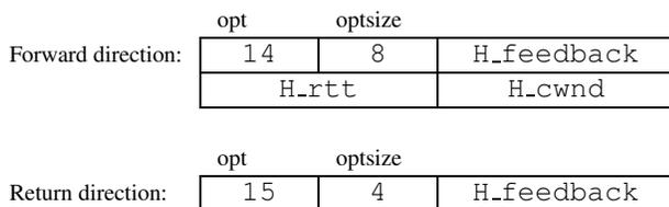
Fig. 1. XCP option formats in both directions
