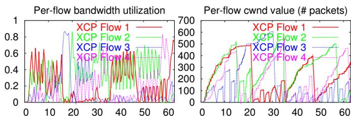
Fig. 18. XCP fails to converge (case 2)
