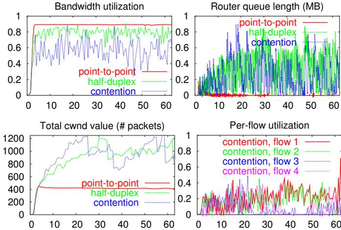
Fig. 10. XCP performances with different link environment.
