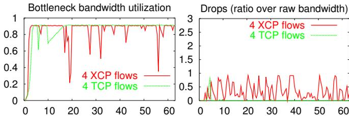
Fig. 15. XCP and TCP performance in the first experiment
