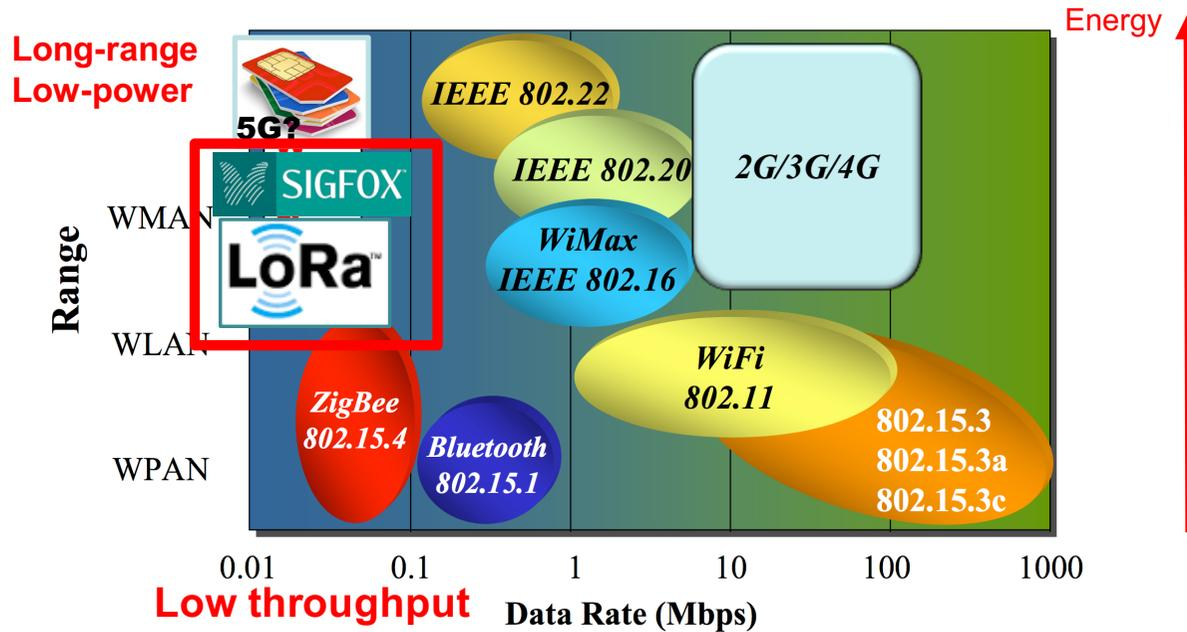
Semtech's LoRa provides low-power long-range transmission enabling several years of operation on batteries
