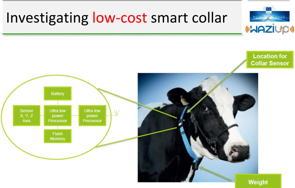
Smart collar unit around the neck of the cow which comprises a 3-axis accelerometer, processor, low power ZigBee wireless interface and two AA batteries.
