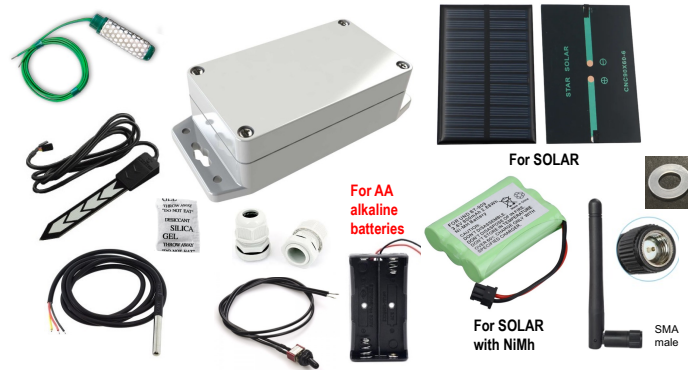
Fig. 2. Off-the-shelf integration: the device’s components, including sensors, can be chosen and obtained separately and independently, thus improving flexibility.
