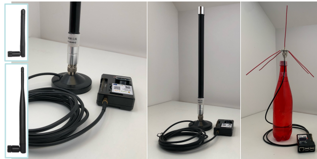
Fig. 6. Indoor higher-gain antennas at the gateway improving coverage.
