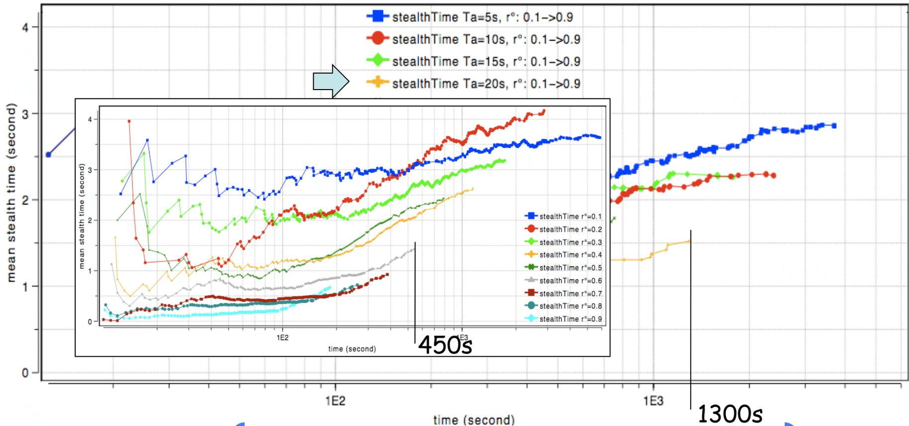
SENSOR NODES START AT 0.1 THEN INCREASE TO 0.9 IF ALERTED (BY INTRUDERS OR NEIGHBORS) AND STAY ALERTED FOR TA SECONDS
