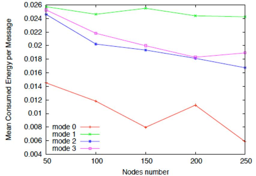
Fig. 7. Mean consumed energy per received packet
