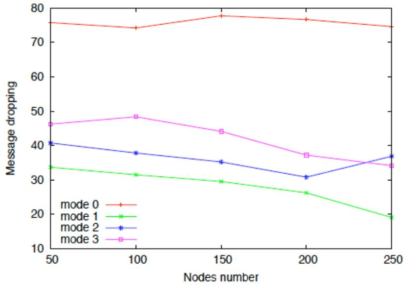
Fig. 4. Message dropping rate at sensor queues
