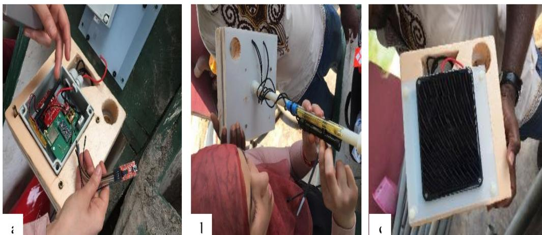
Figure 1: Assembling of the device part on site. (a) Electronic parts in a sealed waterproof box. (b) Sensors along a tube. (c) Solar panel on the top of the device.
