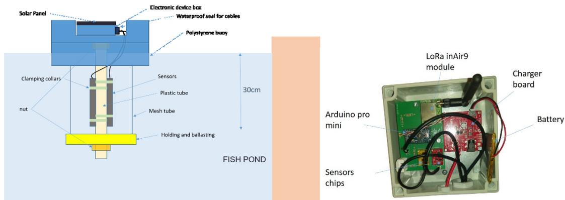
Figure 3: (a) Schema of the first deployed prototype for aquaculture water monitoring in WAZIUP project.
