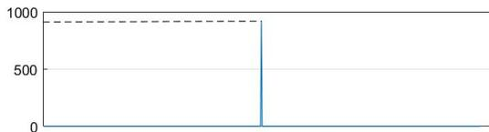
**Figure 4: FFT of 3 Coded chirps at 128.  $SF = 8$ .**
