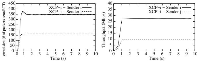
Fig. 8.  $cwnd$  and throughput in the merge scenario
