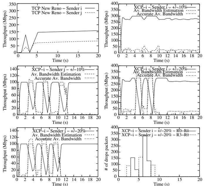
Fig. 13. Top: throughput for TCP (left), XCP-i - Sender i - 10% (right). Middle: throughput for XCP-i - Sender j - 10% (left), XCP-i - Sender i - 20% (right). Bottom: throughput for XCP-i - Sender j - 20%, packet losses XCP-i - 20% (right).
