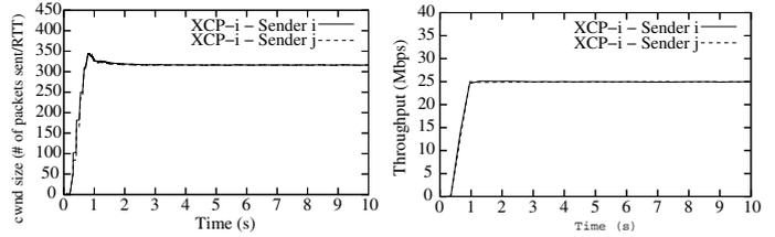
Fig. 12.  $cwnd$  and throughput in the fork scenario
