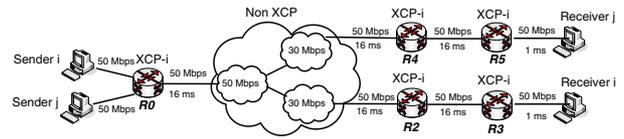
Fig. 11. 1 non-XCP queue shared by XCP-capable downstream nodes
