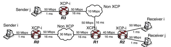
Fig. 7. 2 upstream non-XCP queues,  $\Sigma input\_capacity = output\_capacity$
