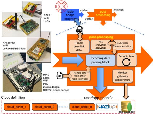
Fig. 3. Modular and versatile low-cost gateway
