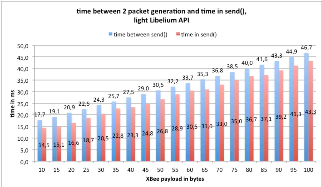
Figure 27: time between 2 packet generation and time in send(), light Libelium API
