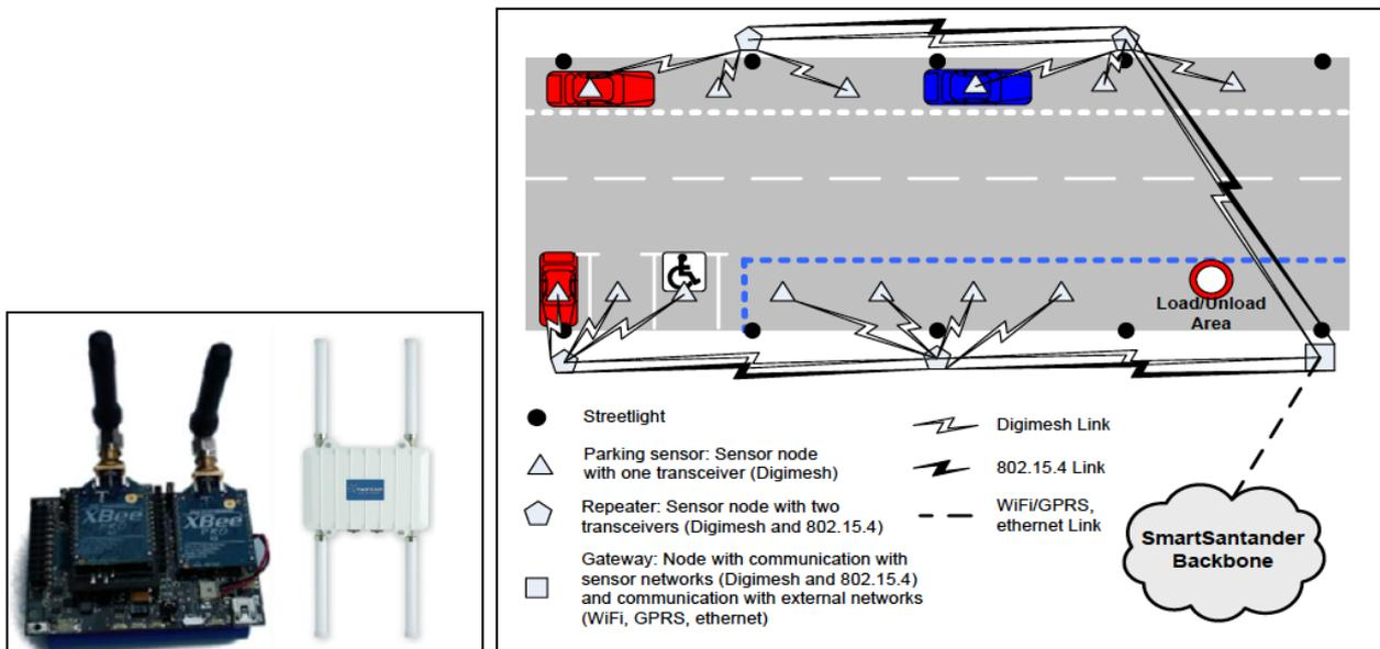
Figure 2: Left: Deployed IoT node and gateway. Right: Communications between IoT nodes and gateways
