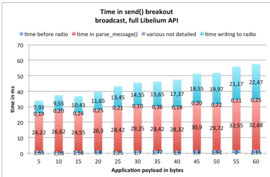
Figure 29: time in `send()` breakout, DigiMesh broadcast, full Libelium API
