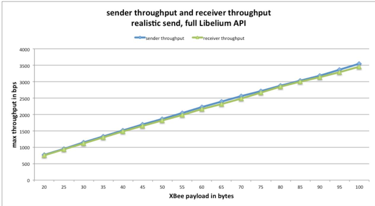
Figure 43: sender throughput and receiver throughput, sender uses full Libelium API
