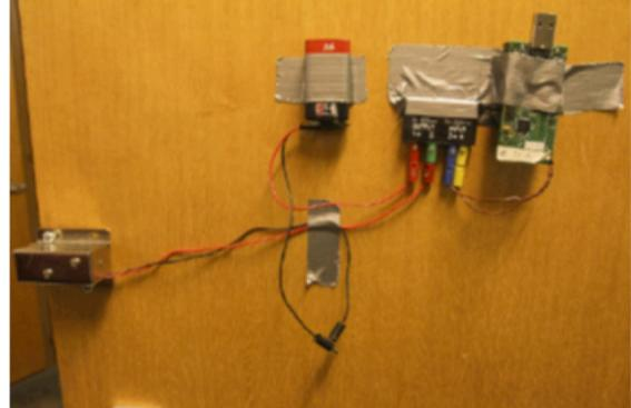
*NFC Reader for User Identification (left) – TelosB mote activating/deactivating a door lock (right)*
