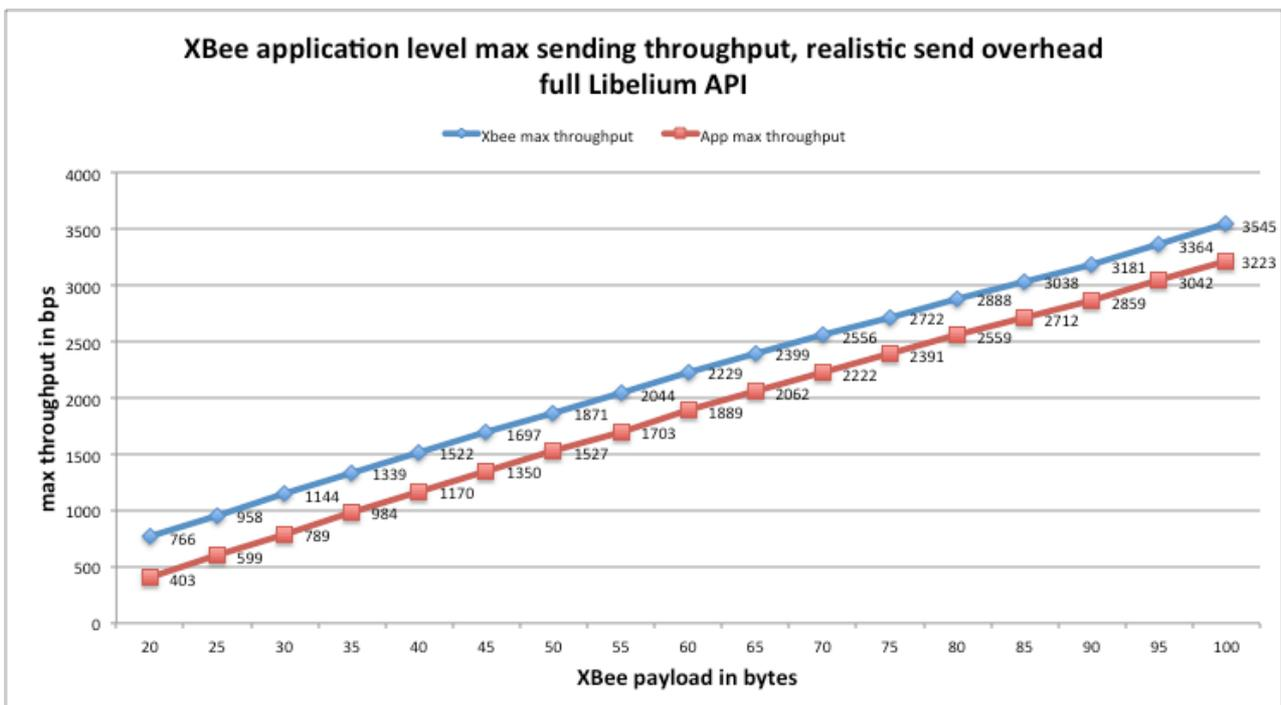
Figure 20: XBee app. level max sending throughput under realistic send overhead, full Libelium API
