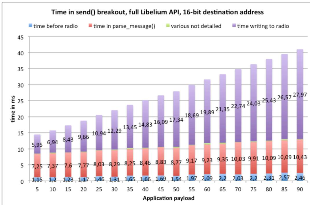
Figure 38: time in send() breakout, full Libelium API, 16-bit destination address
