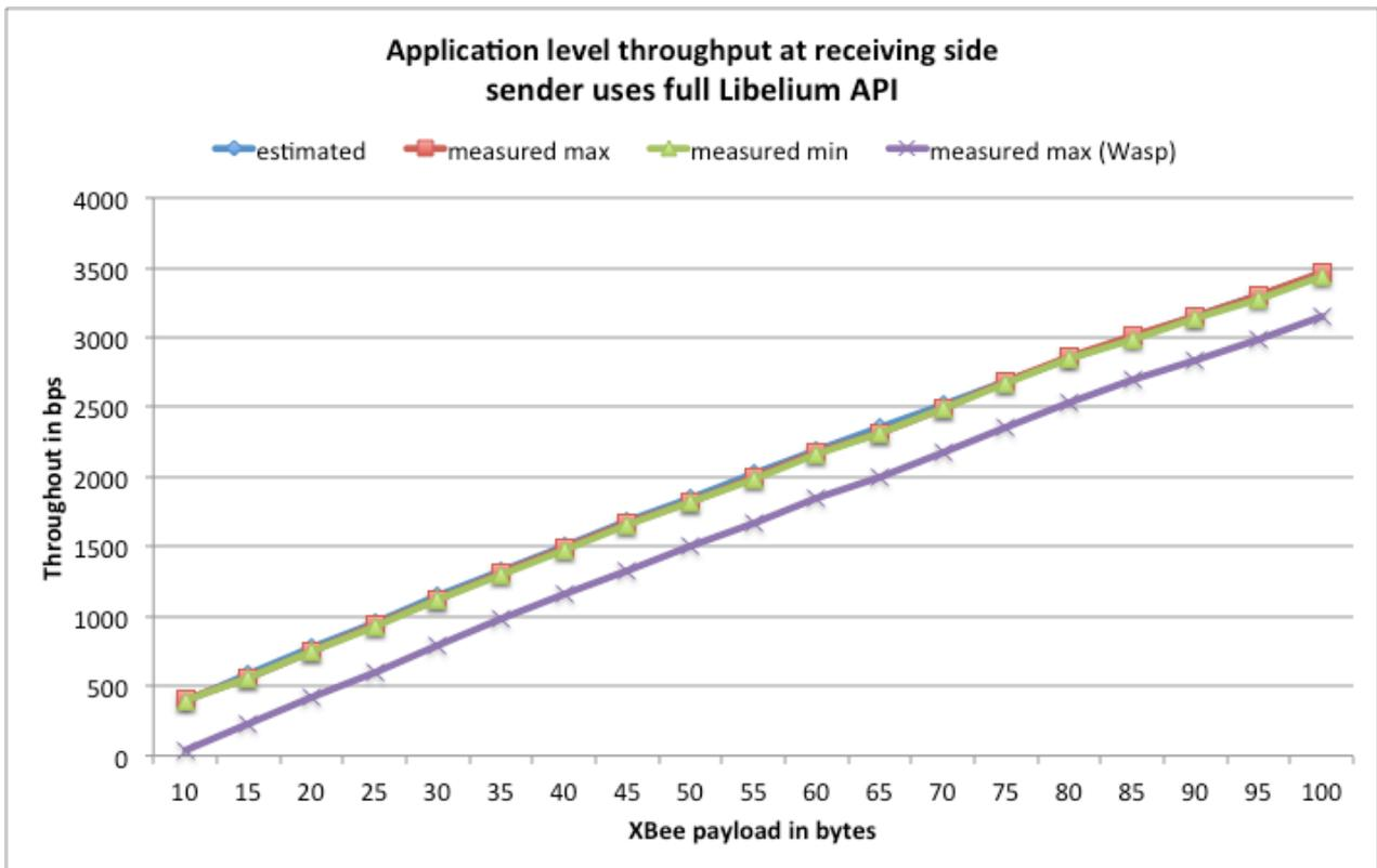
Figure 42: Application level throughput at receiving side, sender uses full Libelium API
