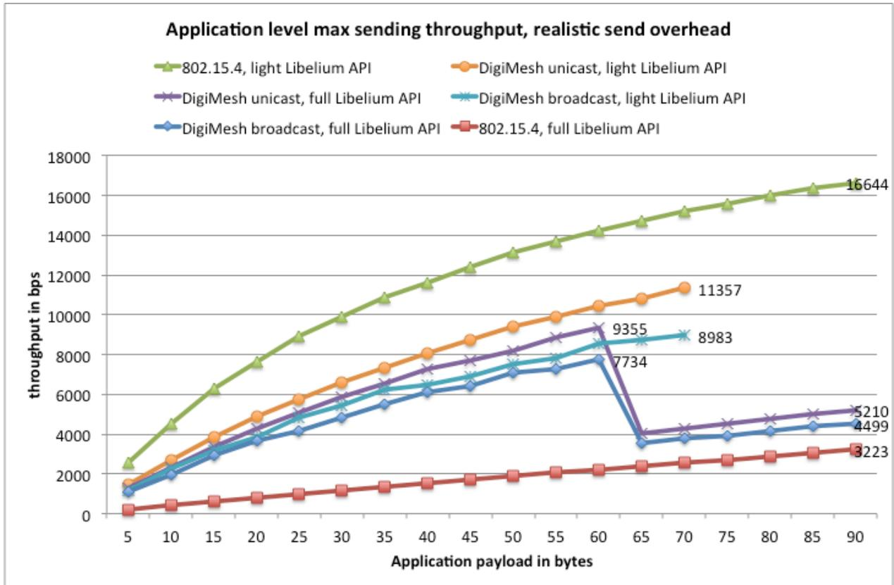
Figure 37: comparison of application level max sending throughput
