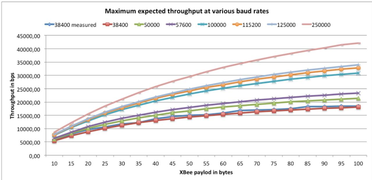
Figure 48: maximum expected sending throughput at various baud rates
