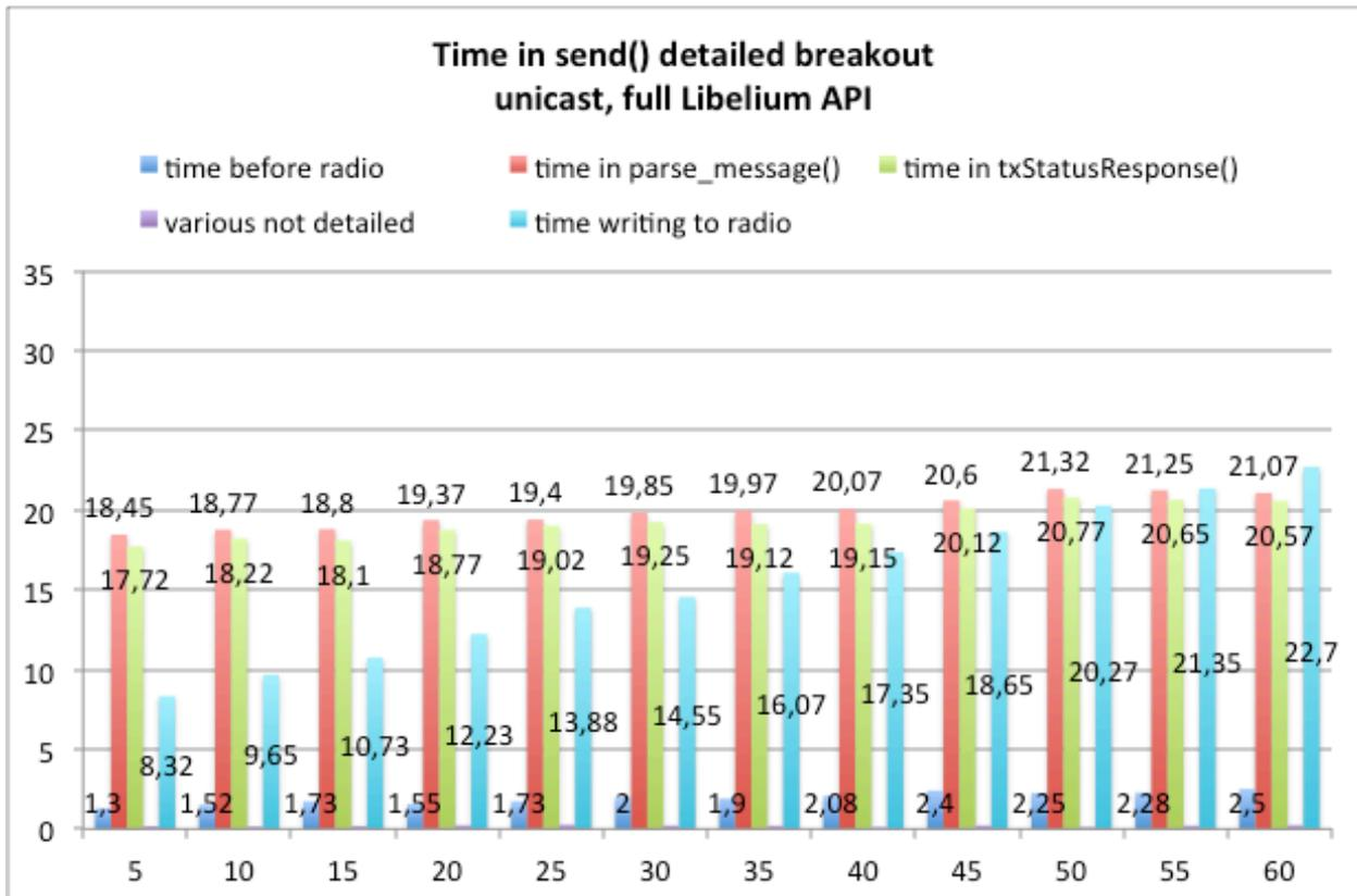
Figure 33: time in send() detailed breakout, DigiMesh unicast, full Libelium API
