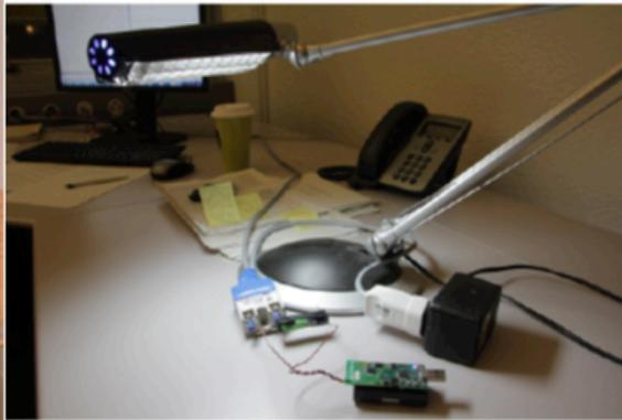
*Fire alarm system including siren and light (left) – Desk lamp controlled by a TelosB mote (right).*
