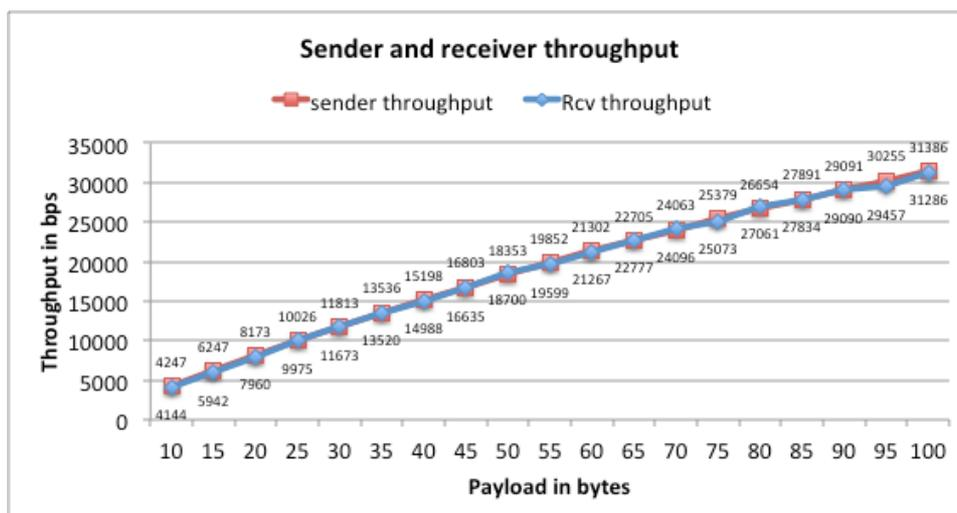
Figure 69: maximum sending throughput for various payload
