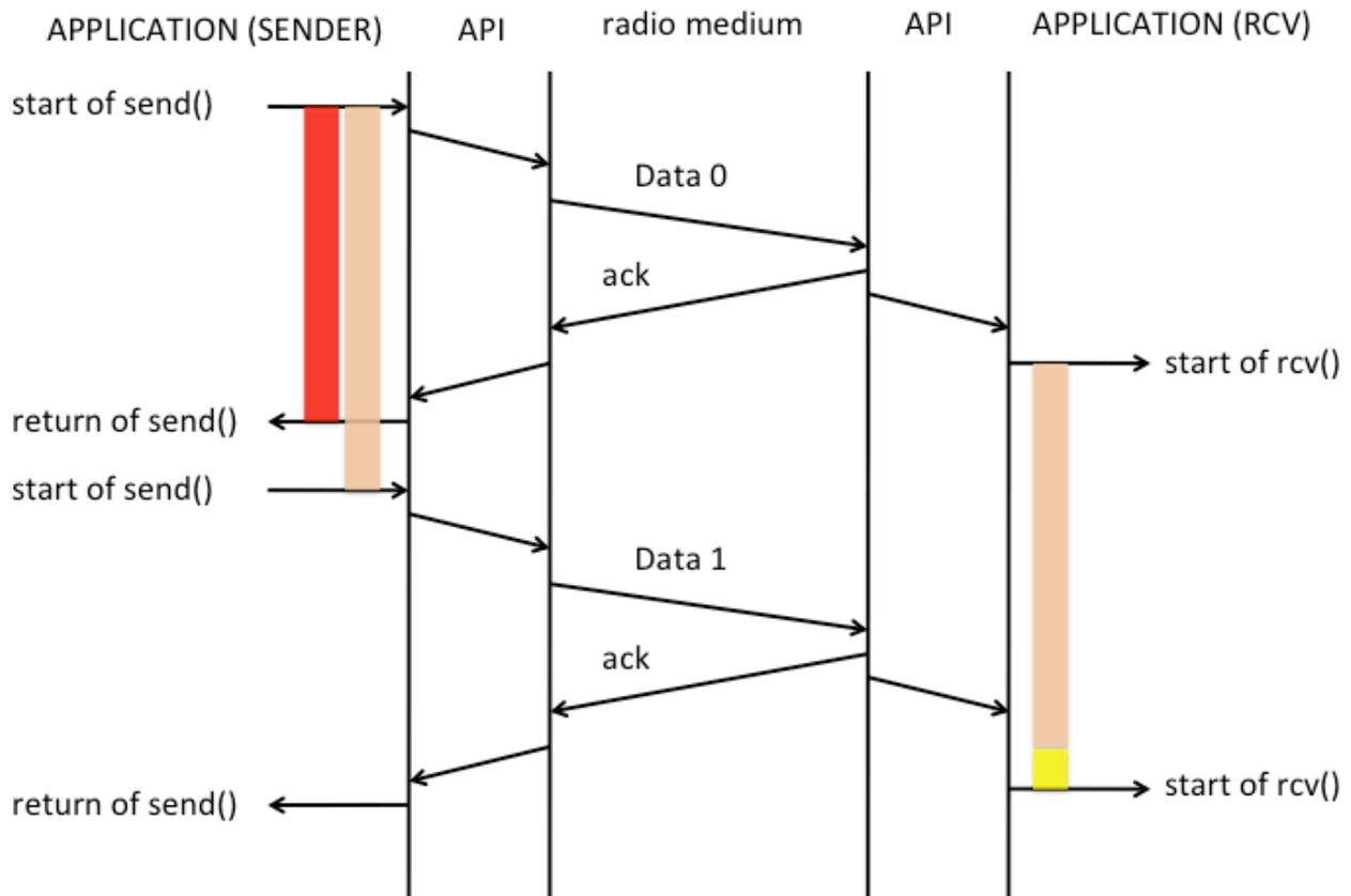
Figure 13: Timing of a sending process
