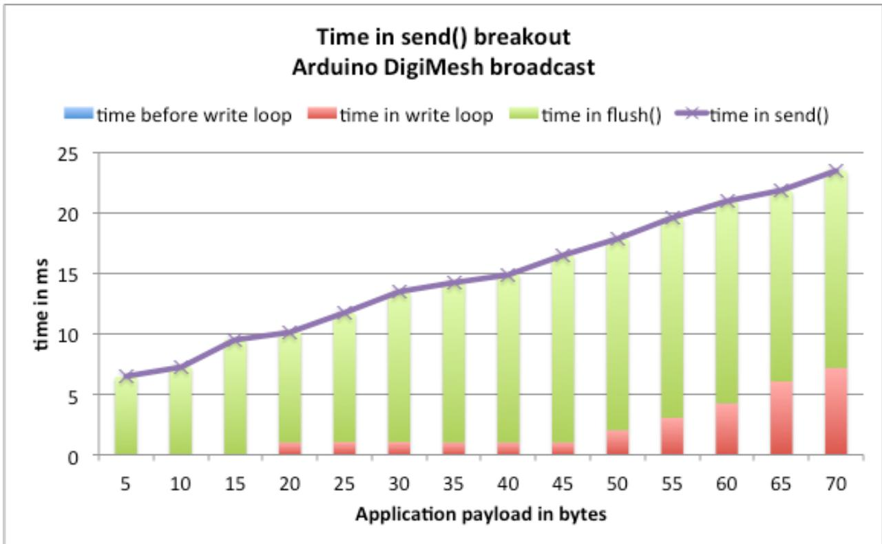
Figure 54: time in send() breakout, Arduino DigiMesh broadcast
