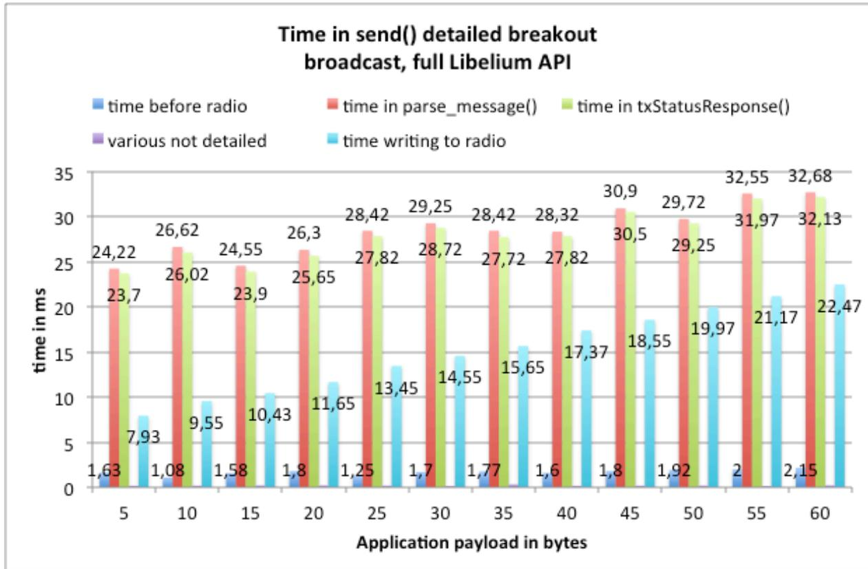
Figure 30: time in `send()` detailed breakout, DigiMesh broadcast, full Libelium API
