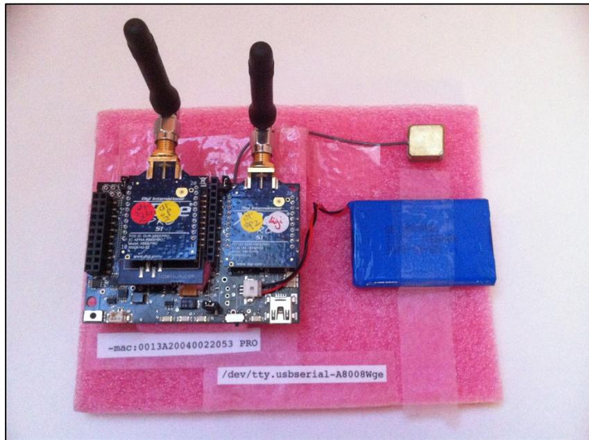
Figure 5: WaspMote with 2 radio modules that reproduces an IoT node in the SmartSantander network
