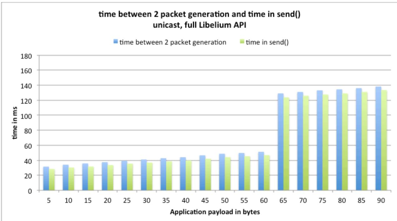
Figure 34: time between 2 packet generation and time in send(), DigiMesh unicast, full Libelium API
