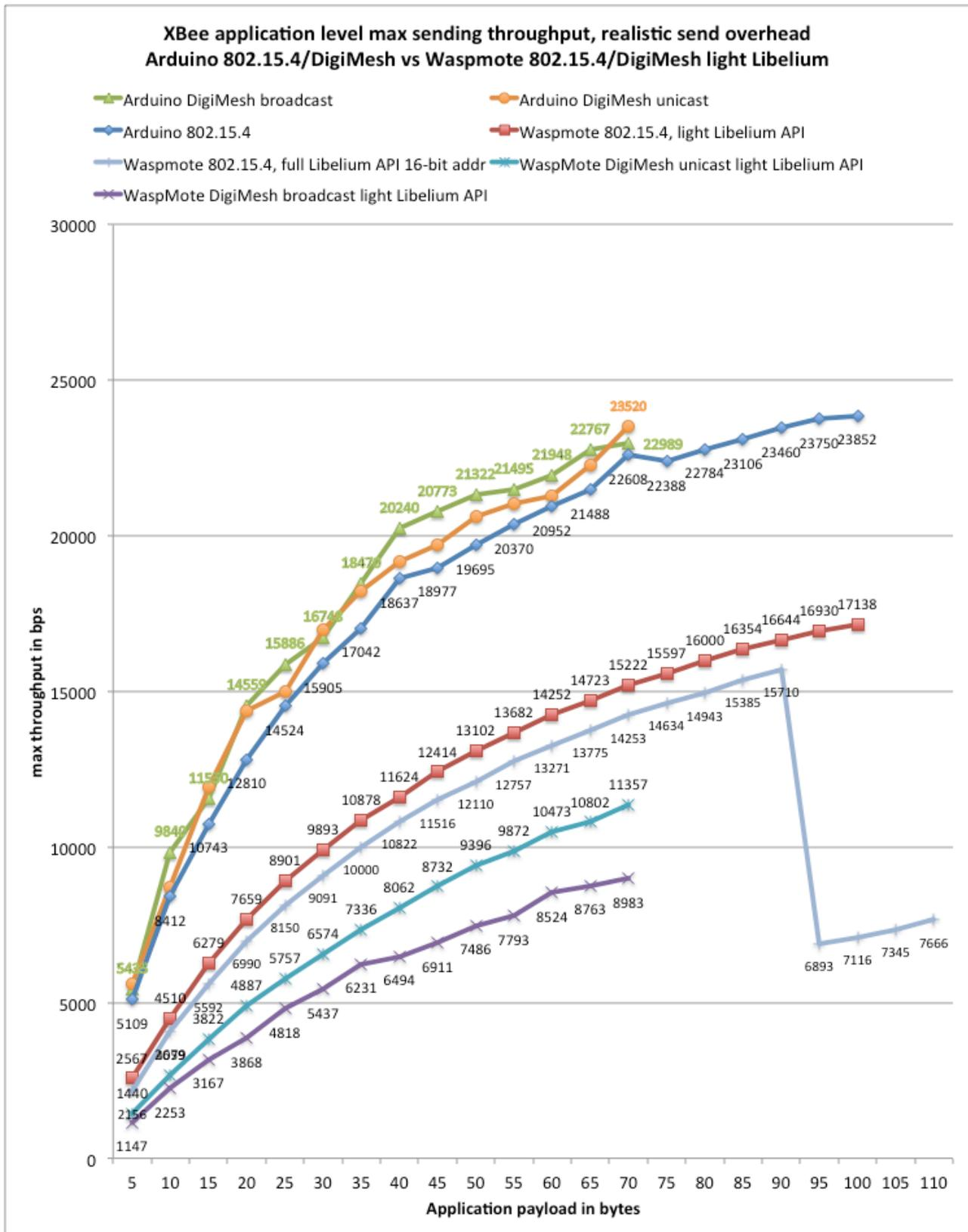
Figure 56: application level maximum sending throughput for various hardware and communication API
