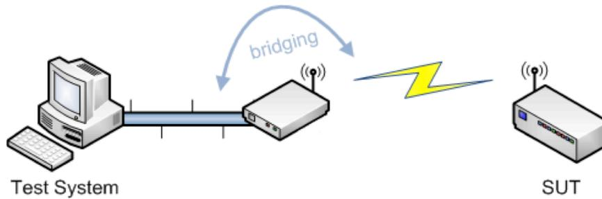
Figure 8: Communication via IEEE802.15.4 adaptation hardware
