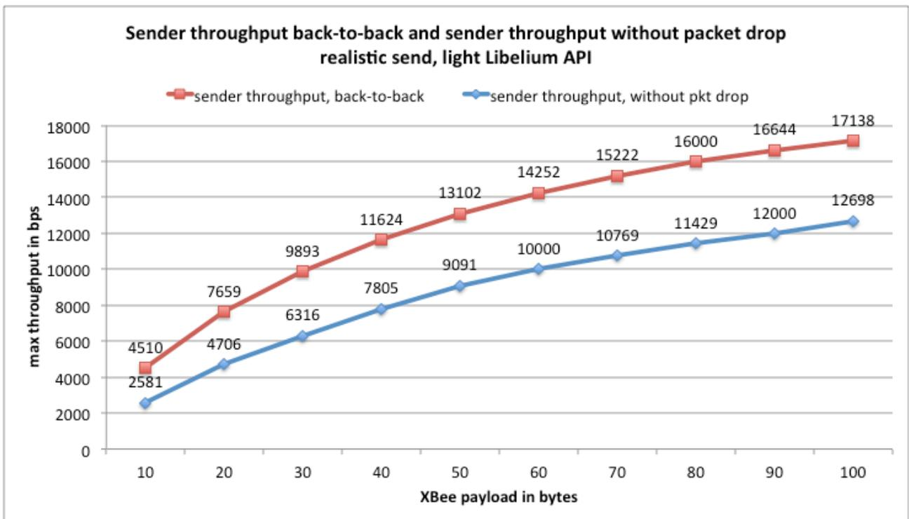
Figure 45: sender throughput back-to-back and receiver throughput, sender uses light Libelium API
