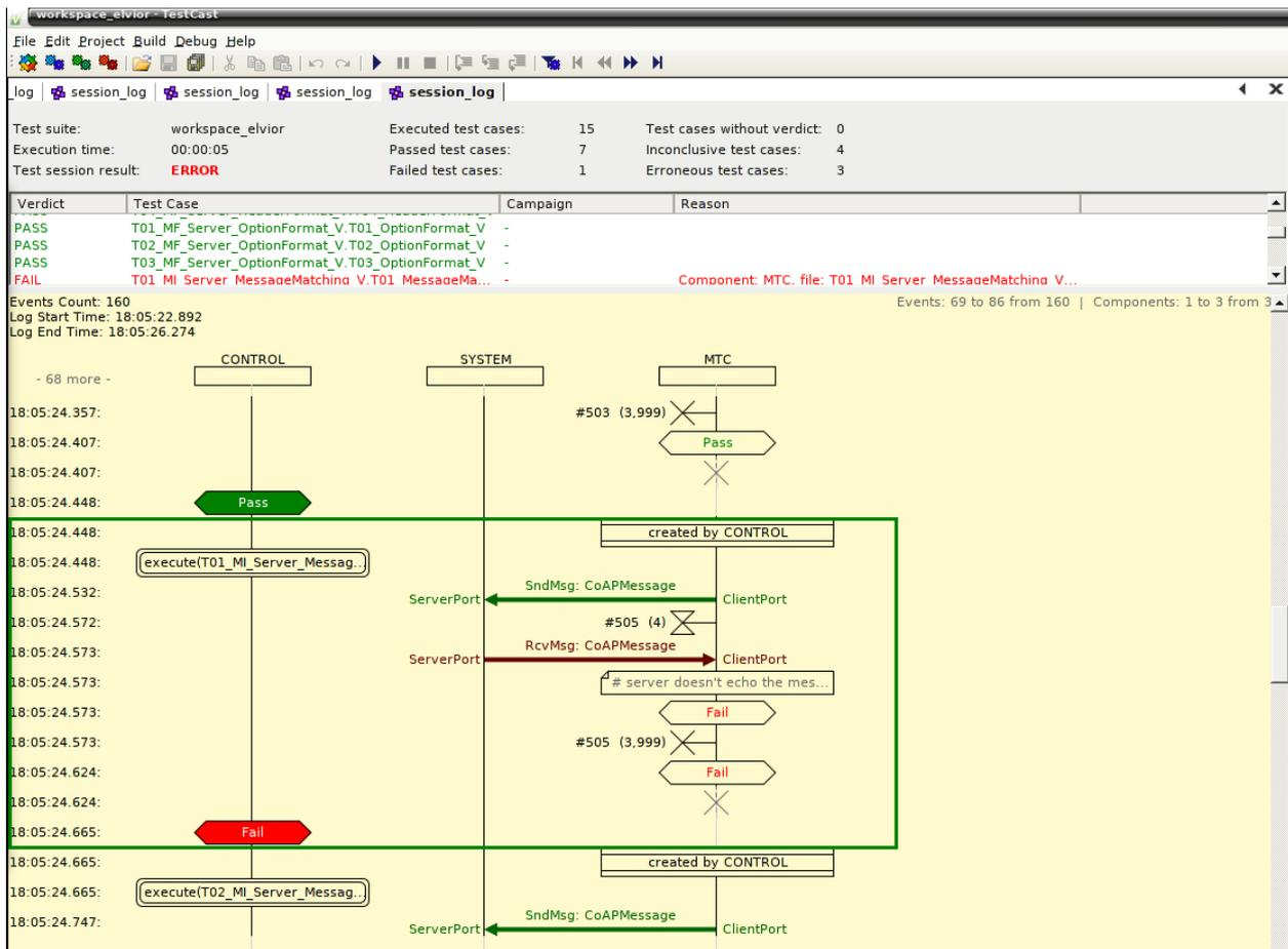
Figure 10: Example of conformance testcase execution
