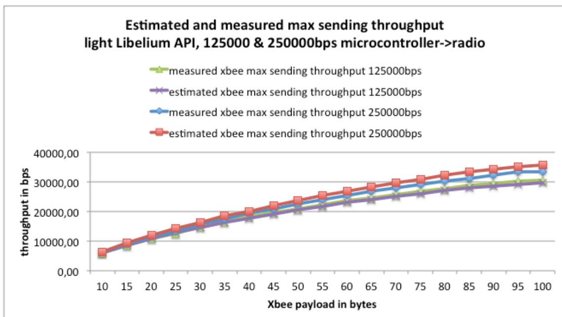
Figure 51: estimated and measured sending throughput for data transfer rates of 125000 and 250000
