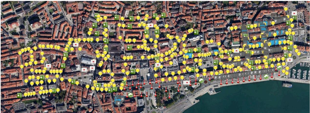
Figure 1: Outdoor parking and Environmental Monitoring deployed architecture
