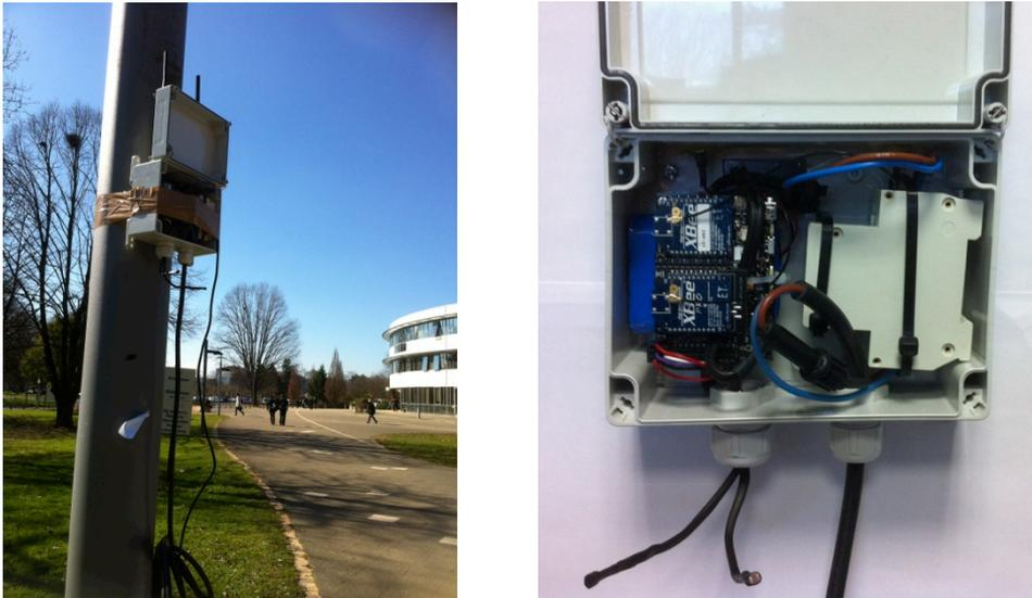
*Figure 60: experimental test, SmartSantander IoT node as traffic generator*
