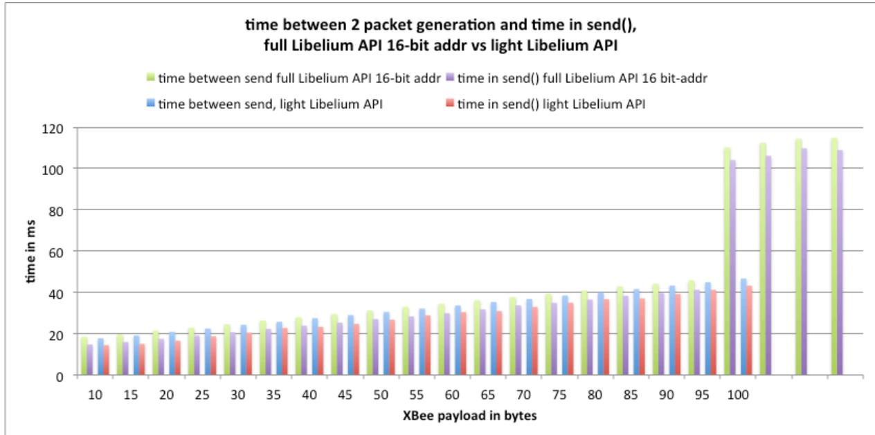
Figure 39: time between 2 packet generation and time in send() for full Libelium API 16-bit address and light Libelium API
