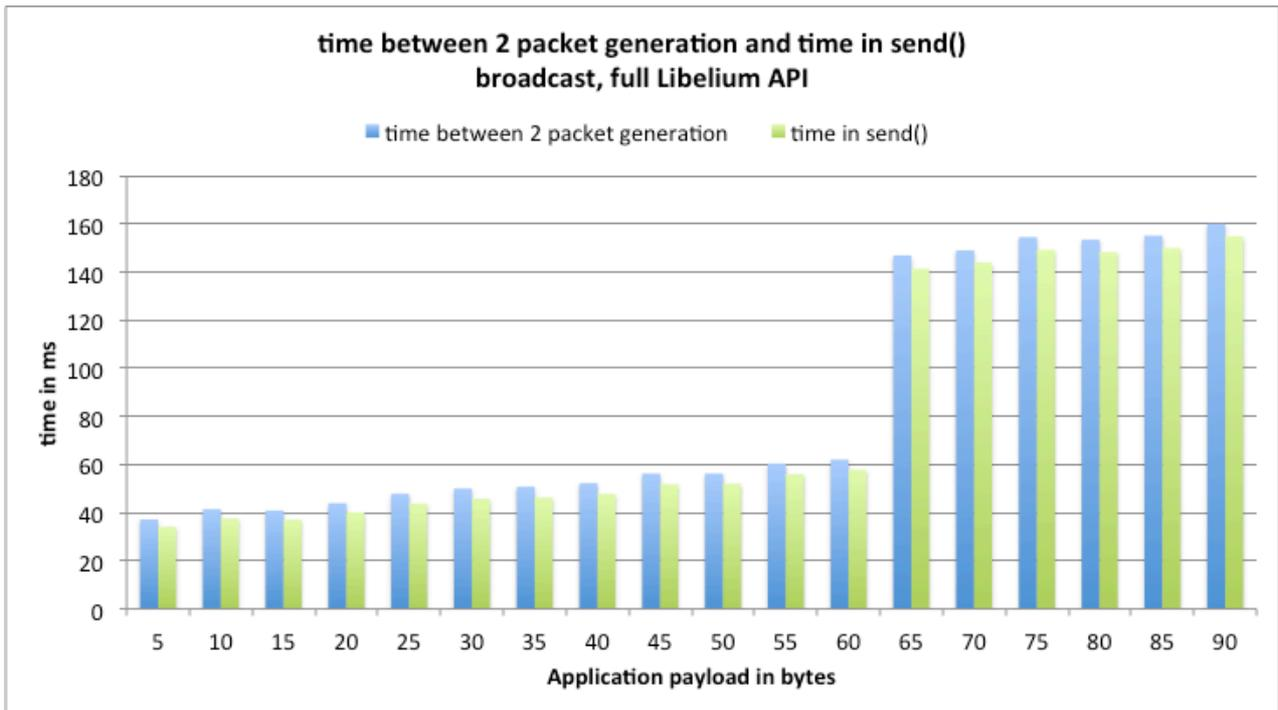
Figure 31: time between 2 packet generation and time in send(), DigiMesh broadcast, full Libelium API
