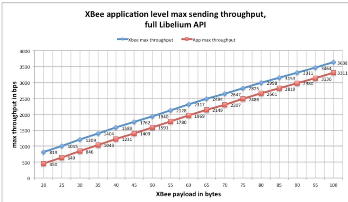
Figure 18: maximum application level max sending throughput, full Libelium API
