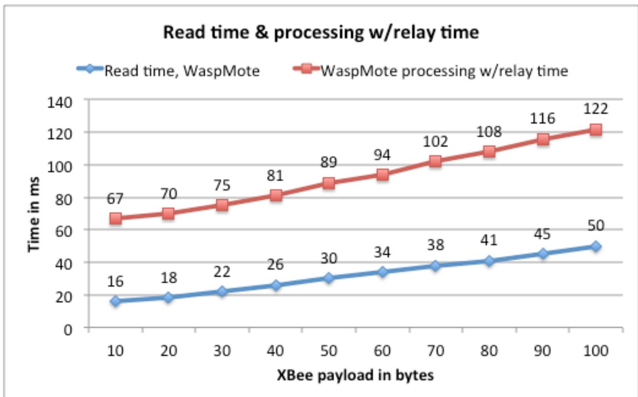
Figure 58: Time to read data from serial (blue) and total processing time w/relay
