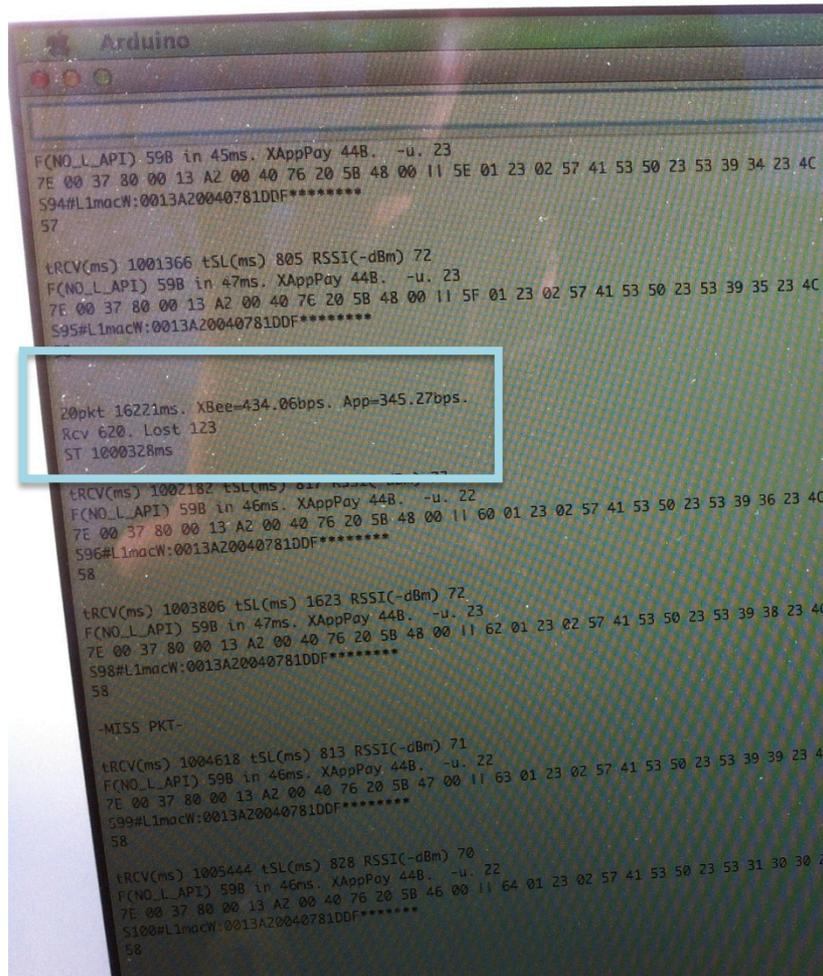
Figure 60: experimental test, traffic generator, final sniffer and relay node
