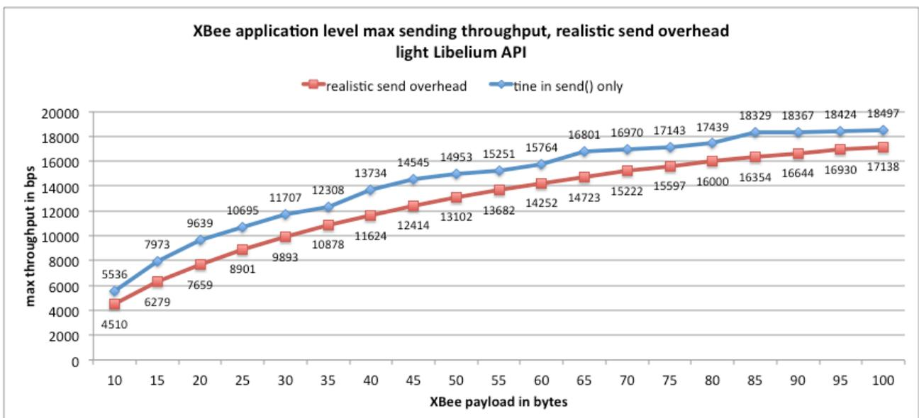
Figure 28: XBee app. level max sending throughput under realistic send overhead, light Libelium API
