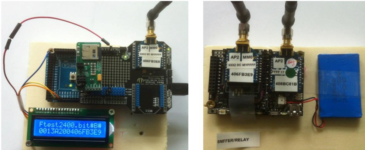
Figure 61: Left: Arduino Mega2560 for sending acoustic data stored in the SD card. Right: A WaspMote relay node
