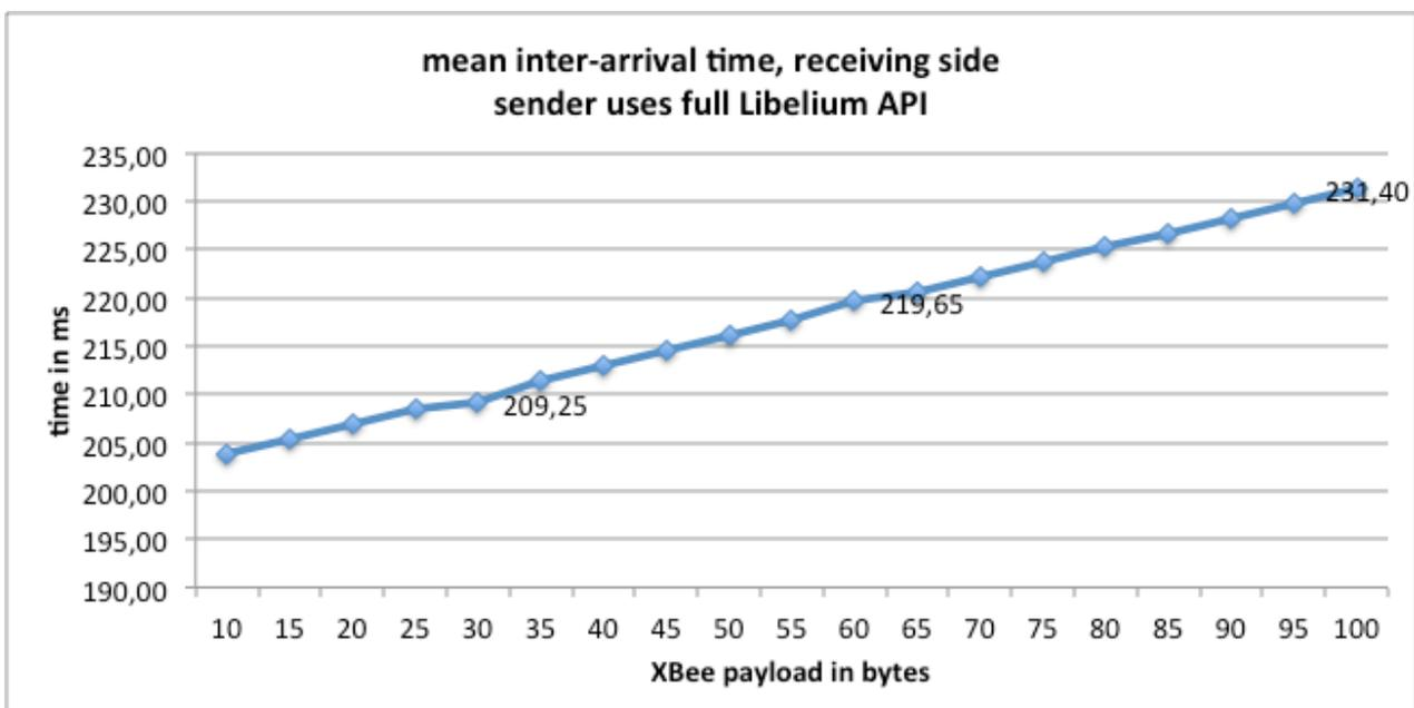
Figure 41: mean inter-arrival time at receiving side
