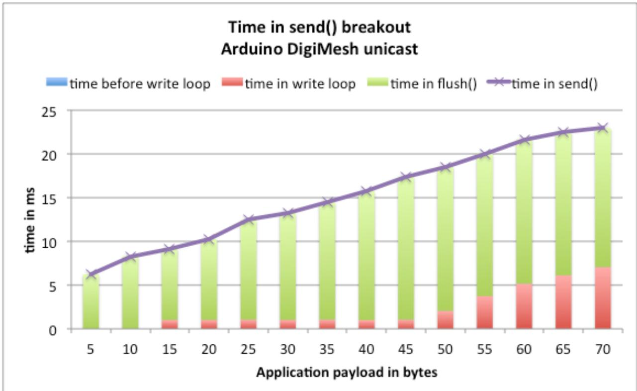
Figure 55: time in send() breakout, Arduino DigiMesh unicast
