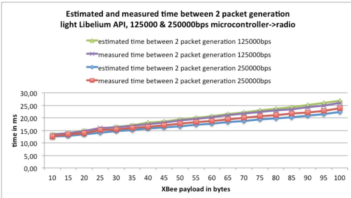
Figure 50: estimated and measured time between 2 packet generation for data transfer rates of 125000 and 250000
