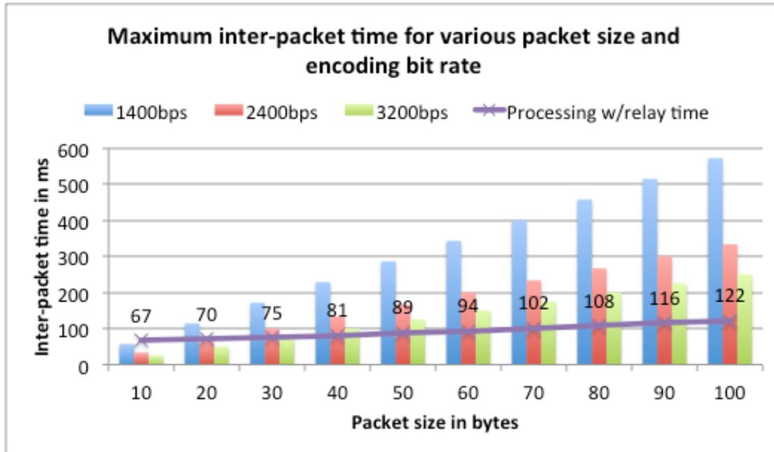
Figure 64: Maximum inter-packet time at various packet size and encoding rate
