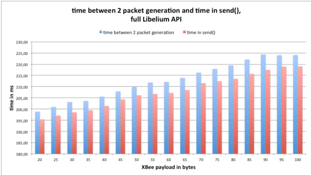
Figure 19: time between 2 packet generation and time in send(), full Libelium API
