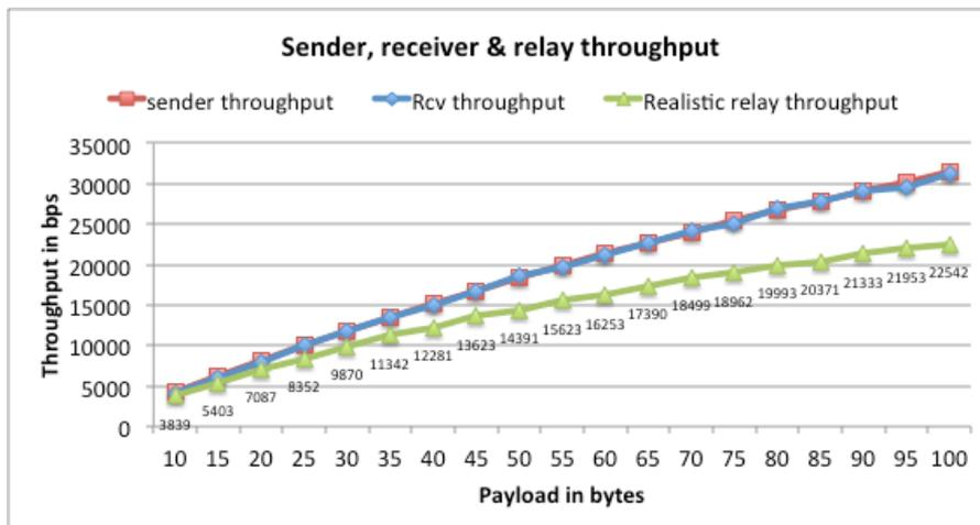
Figure 72: Realistic relay throughput
