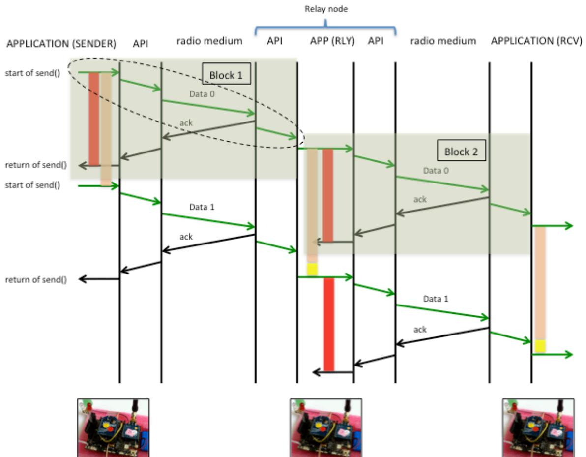
Figure 57: generic relay process, 2-hop with 1 relay node
