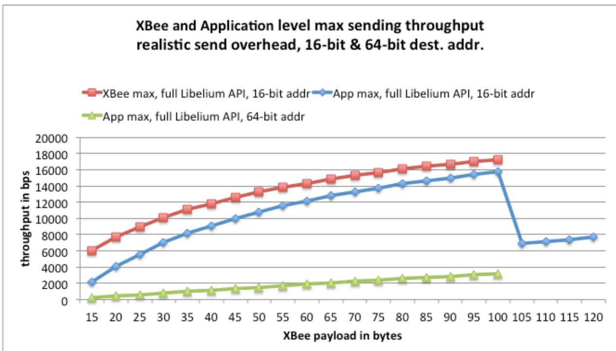
Figure 40: XBee and app. level max. sending throughput, full Libelium 16-bit addr. and light Libelium
