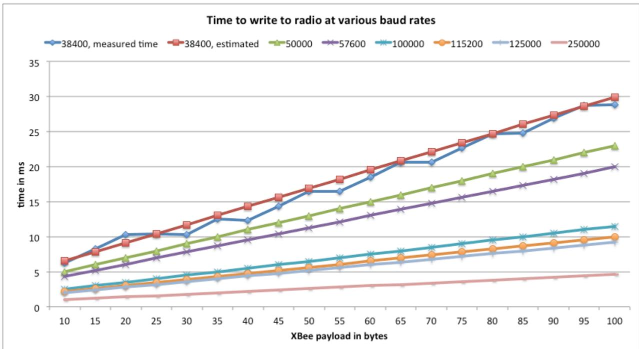
Figure 47: time to write to radio at various baud rates
