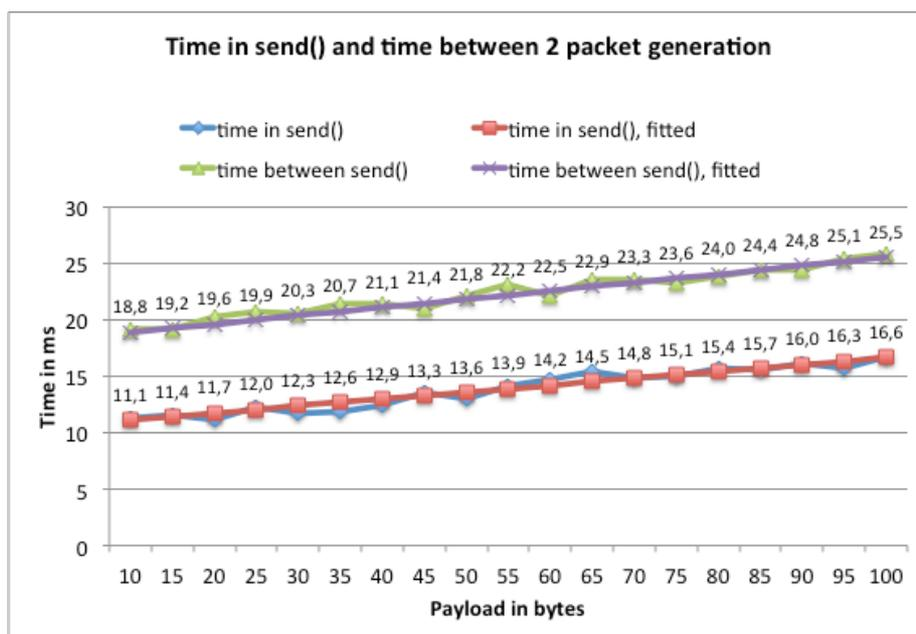
Figure 67: mean time in send() and mean time between 2 packet generation for various payload
