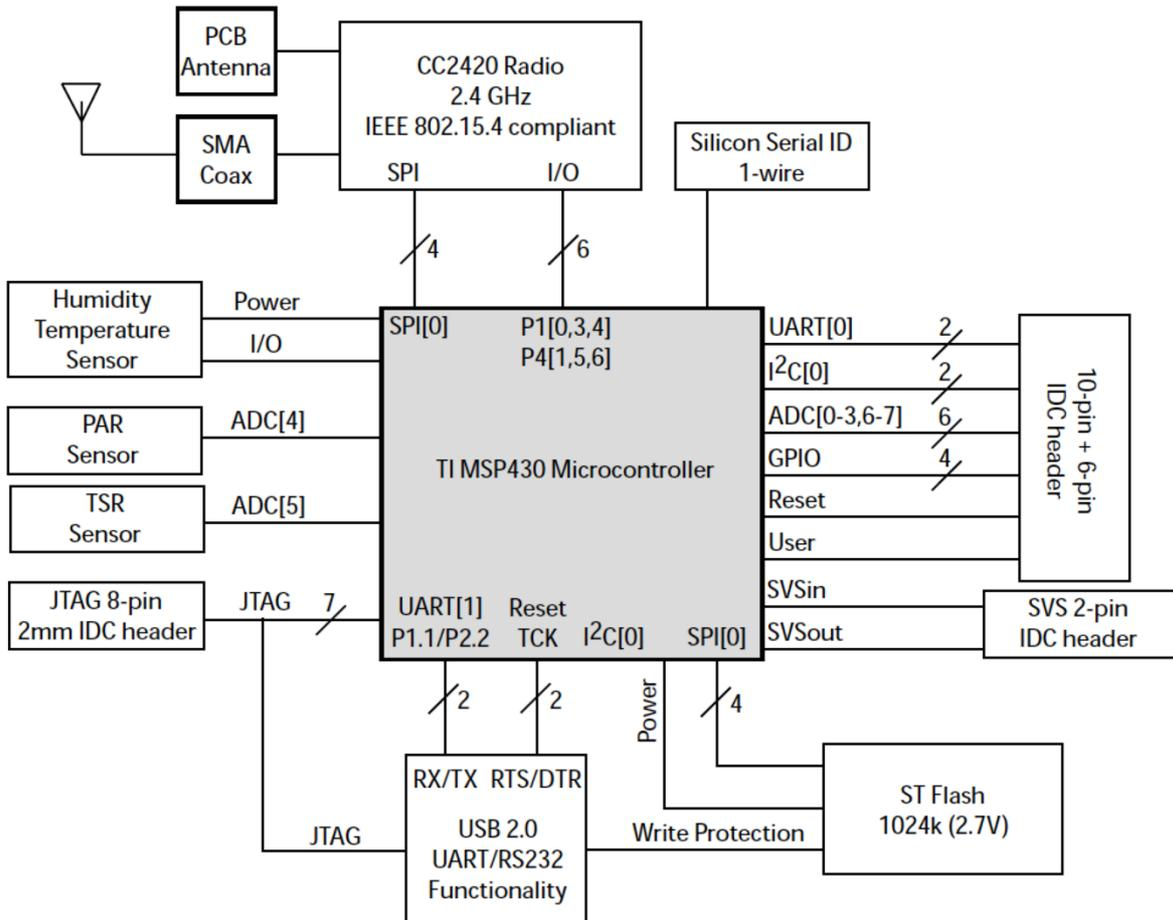
Figure 10a: Functional Block Diagram of the Telos Module, its components, and buses
