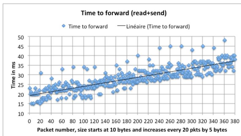
Figure 71: packet read time and packet relay time
