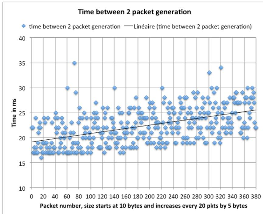
Figure 66: time between 2 packet generation for various payload
