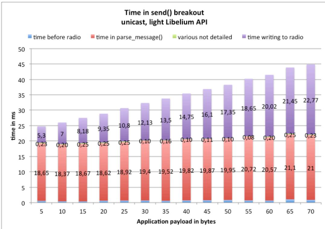
Figure 36: time in send() breakout, DigiMesh unicast, light Libelium API
