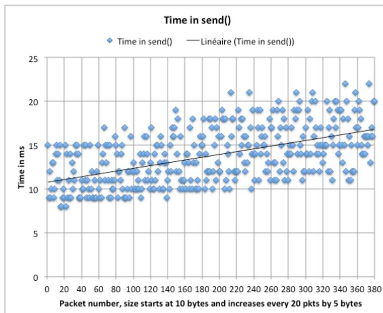
Figure 65: time in send() for various payload
