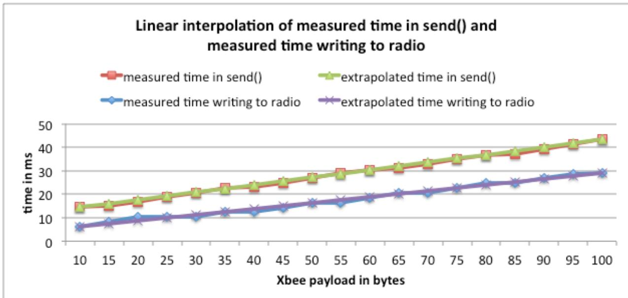
Figure 49: linear interpolation to avoid amplifying measure uncertainty
