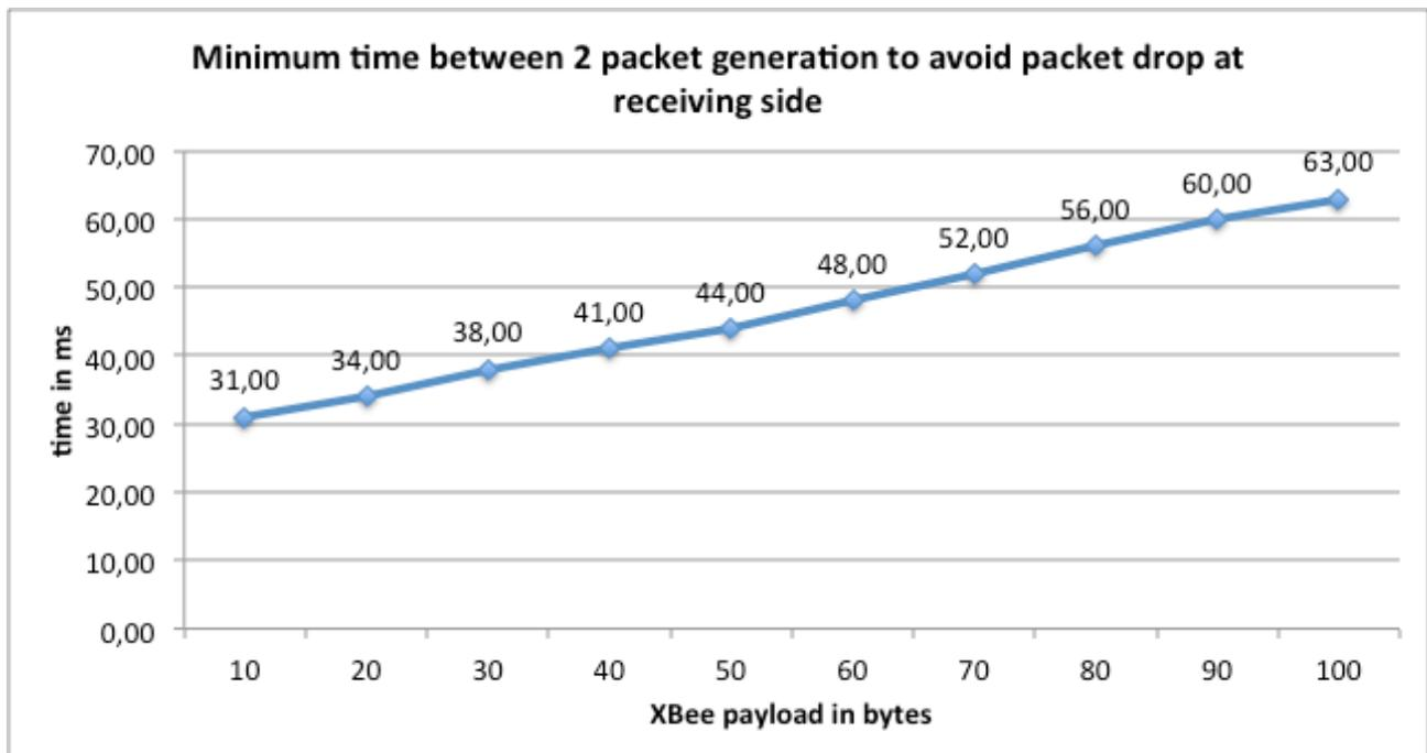
Figure 44: Minimum time between 2 packet generation to avoid packet drop at receiving side
