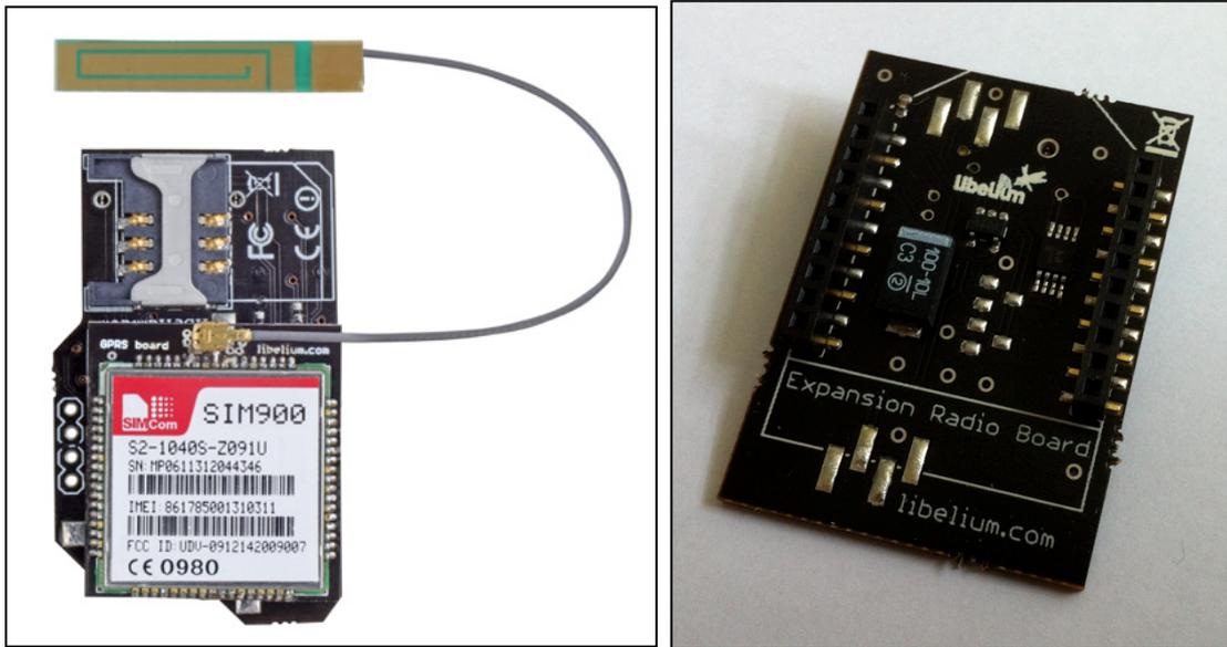
Figure 4: GSM/GPRS module (left), Radio Expansion Board (right)
