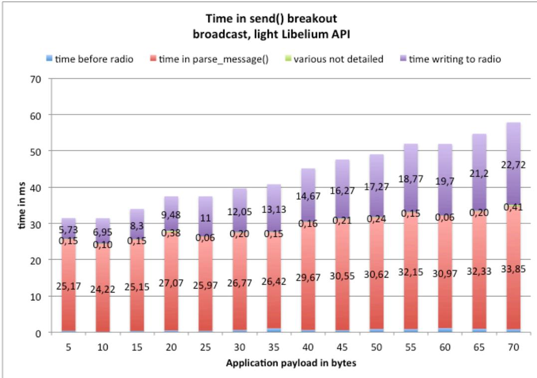
Figure 35: time in send() breakout, DigiMesh broadcast, light Libelium API
