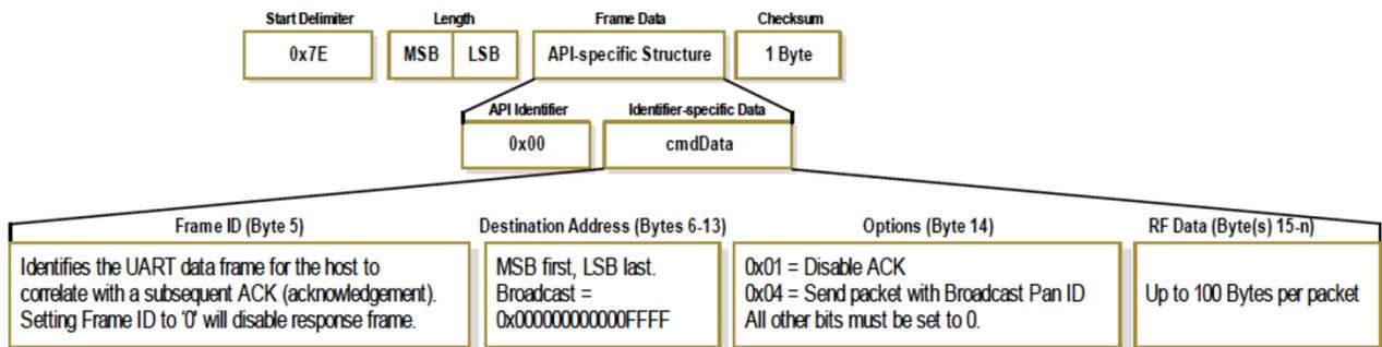
Figure 46: API frame for a transmit request
