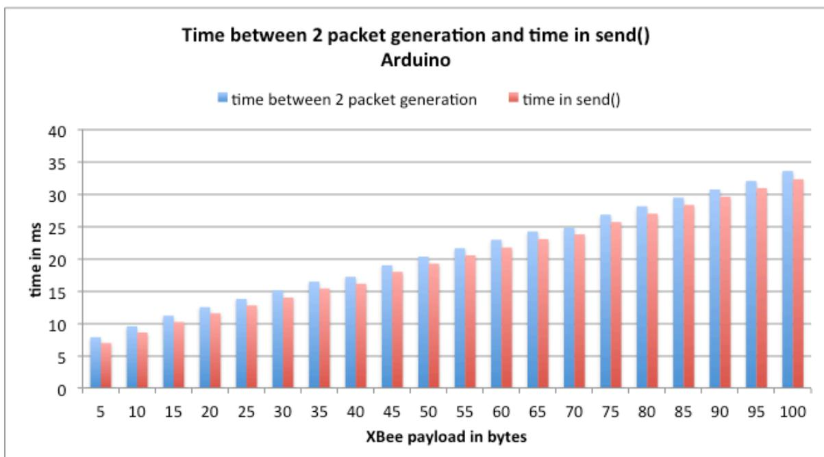
Figure 53: time between 2 packet generation and time in send(), Arduino 802.15.4 module
