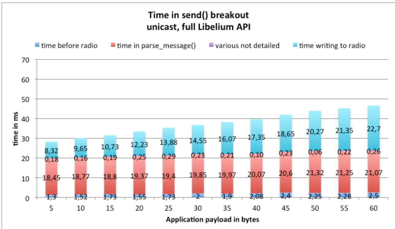
Figure 32: time in send() breakout, DigiMesh unicast, full Libelium API
