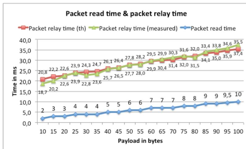
Figure 70: packet read time and packet relay time
