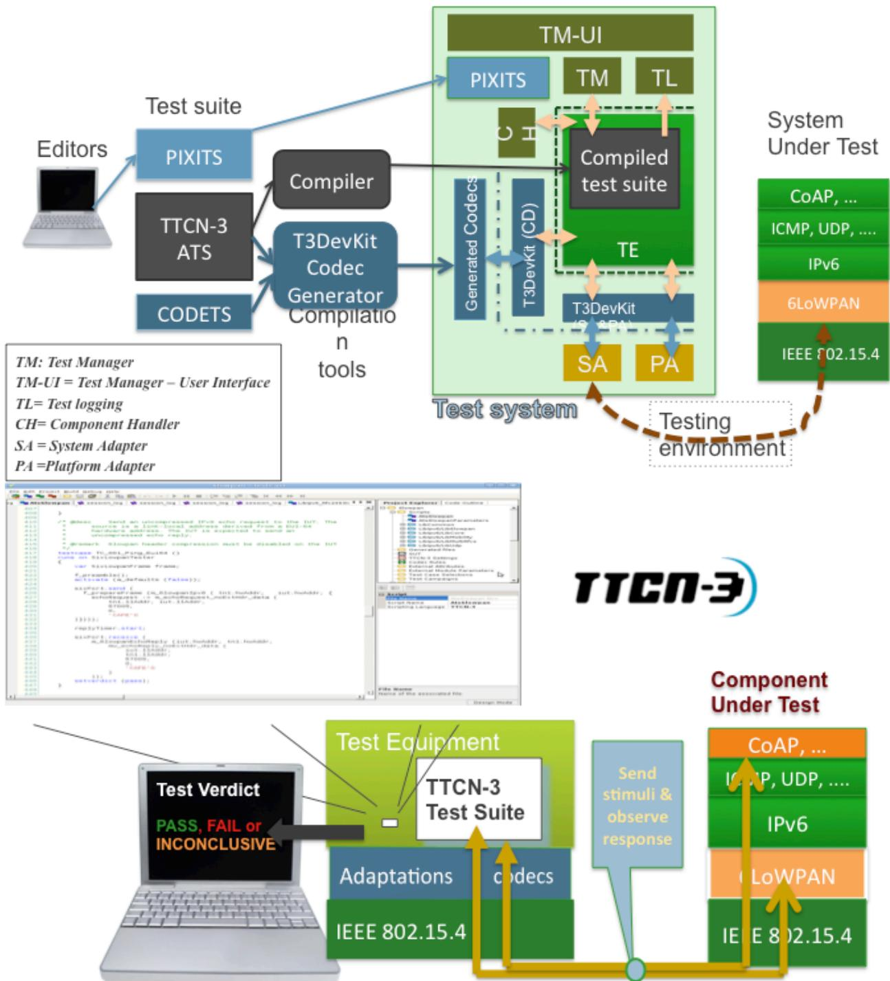
Figure 7: General Architecture of a TTCN-3 test platform
