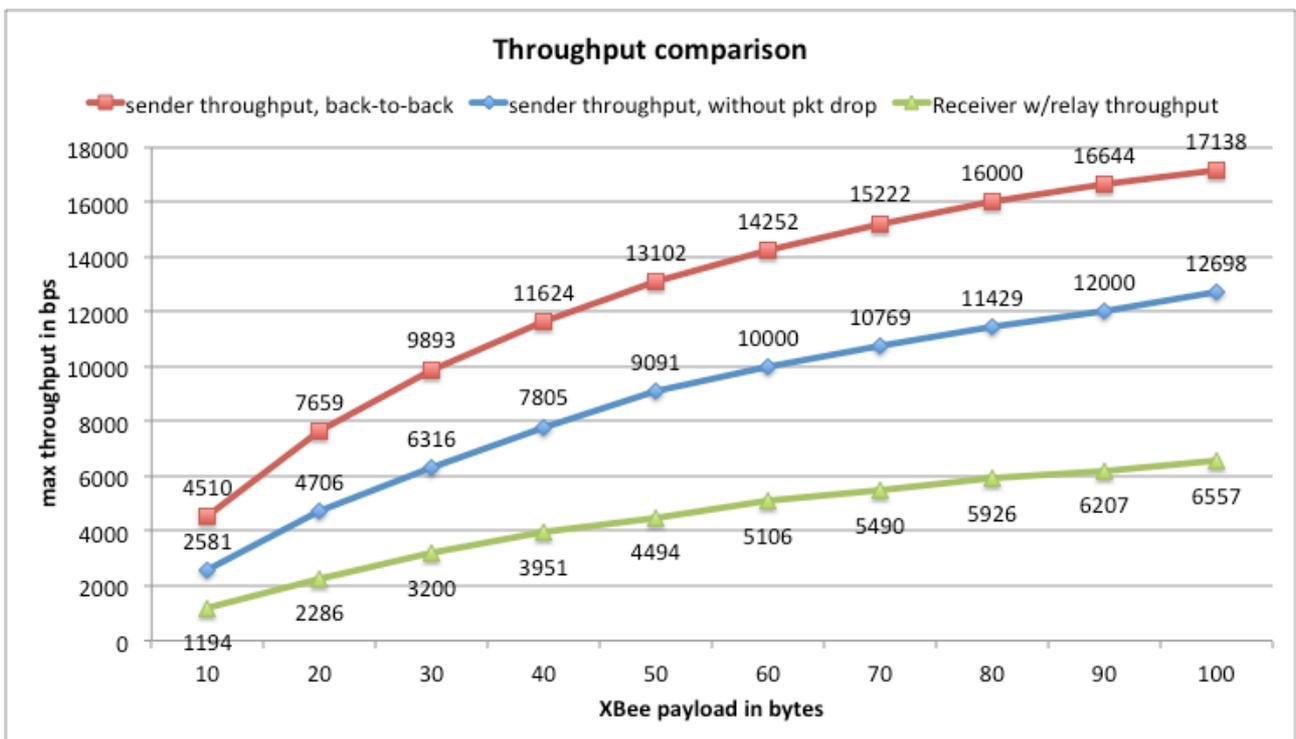
Figure 59: Throughput comparison
