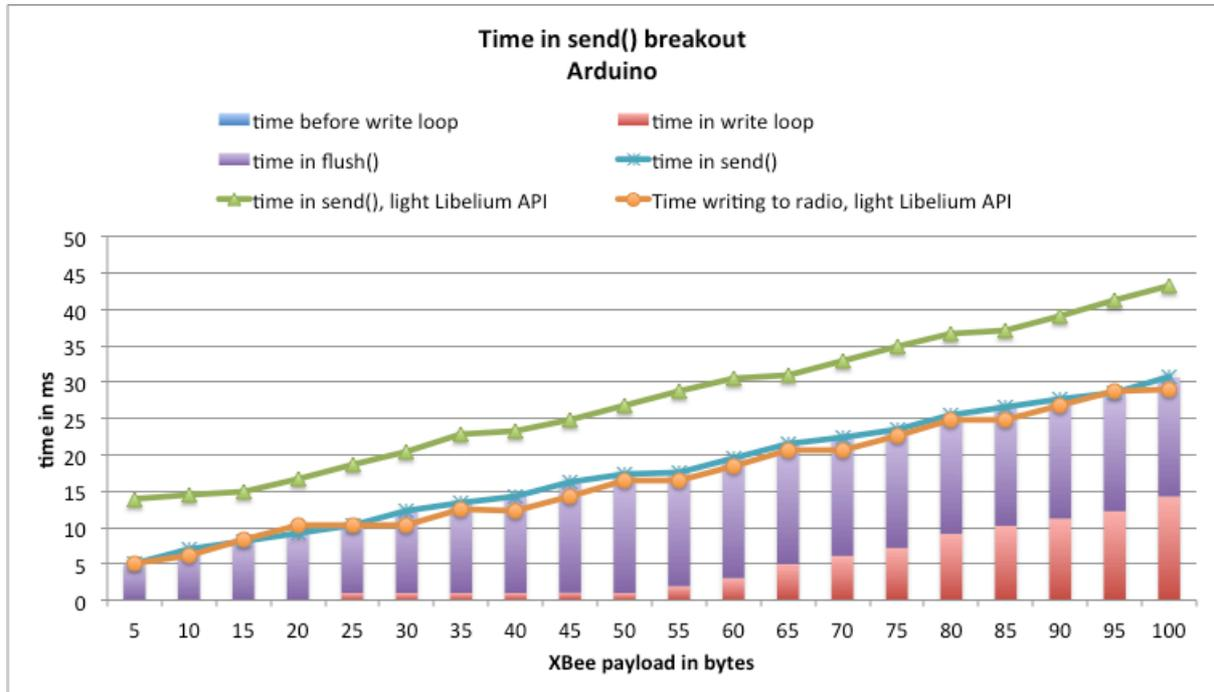
Figure 52: time in send() breakout, Arduino 802.15.4 module
