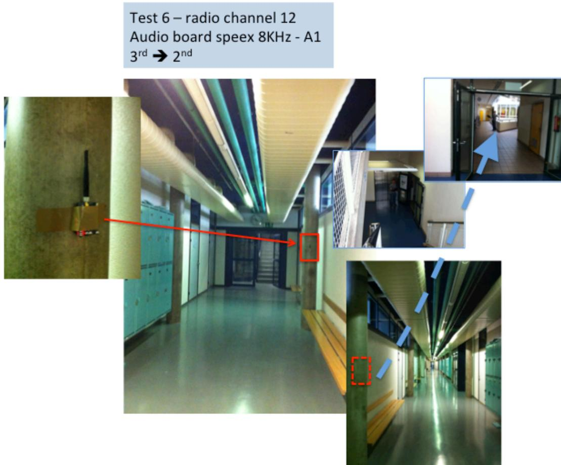
Figure 54 : test#6 in a long corridor of the HEPIA building, receiver in 2nd floor
