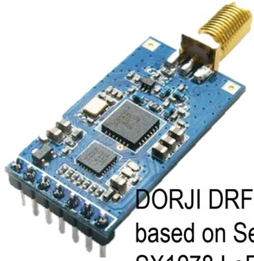
DORJI DRF1278DM is based on Semtech SX1278 LoRa 433MHz
