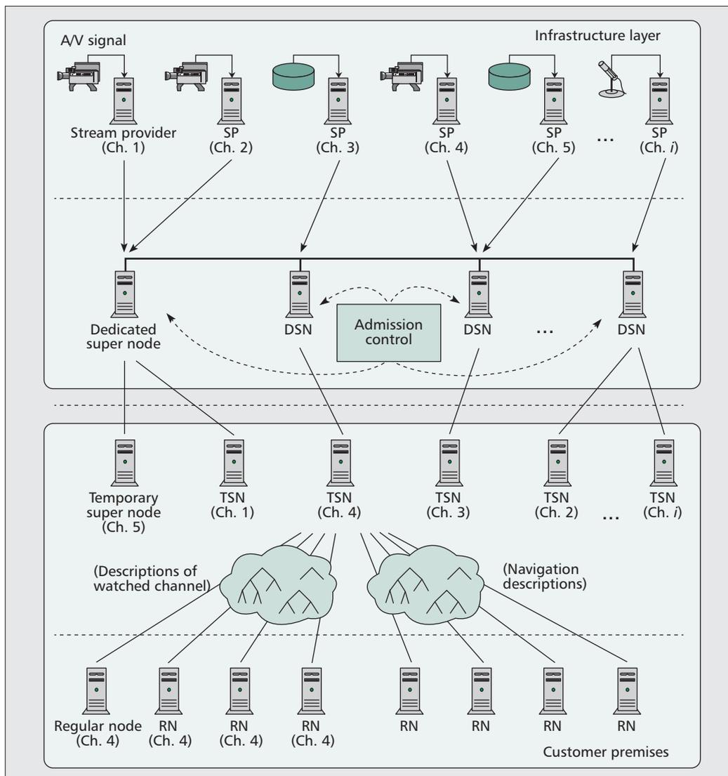
In P2P networks, there are two main approaches to video distribution: tree and mesh. The tree approach, based on multicasting on the application layer, has a distribution structure always ready for transmission. The mesh approach employs connections on demand.
