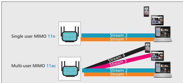
Figure 3. Illustration of MU-MIMO 802.11ac and SU-MIMO 802.11n.
