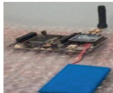
Fig. 1. WSN node architecture and a real Waspmote example.
