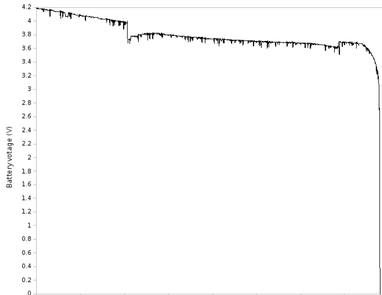
Figure 75: Typical discharging curve for battery
