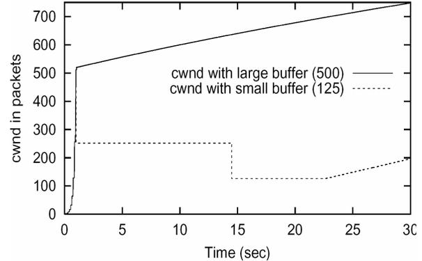
Figure 3. *cwnd* dynamics in NewReno with Hoe's modification
