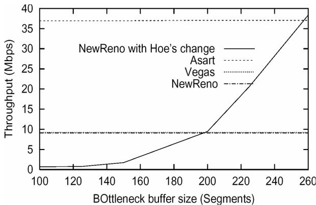
Figure 10. Throughput vs. bottleneck buffer size (first 20 seconds)
