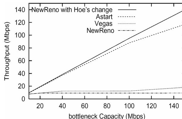
Figure 9. Throughput vs. bottleneck capacity (first 20 seconds)
