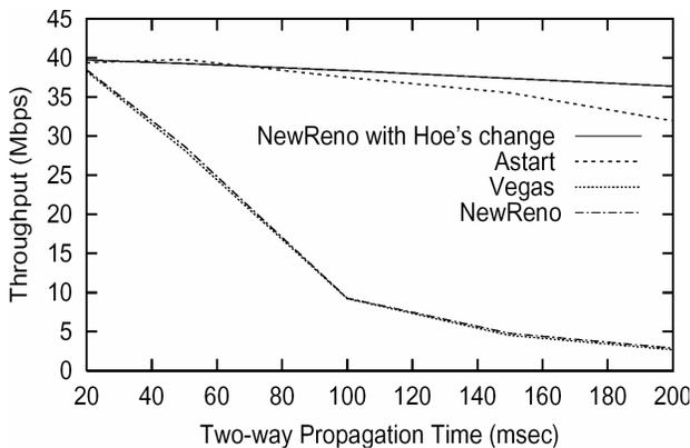
Figure 11. Throughput vs. two-way propagation time (first 20 seconds)
