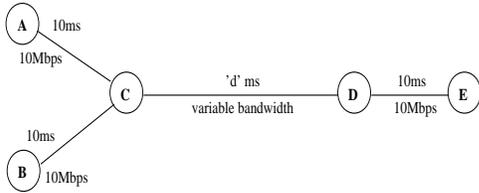
Fig. 2. The Simulation Network with Changing Bandwidth
