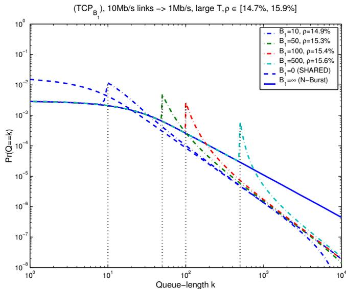
Fig. 5. The queue-length distribution of the  $TCP_{B_1}$  model for  $N = 2$  sources and long Power-Tails: Below the peak at  $k = B_1$ , the distributions is close to the  $N$ -Burst model. After the peak, the queue-length of the  $TCP_{B_1}$  model approaches the distribution of the SHARED model. The model here uses TPT distributed connection sizes with a large number of phases, such that the impact of the truncation is not visible in the plotted range of queue-lengths.
