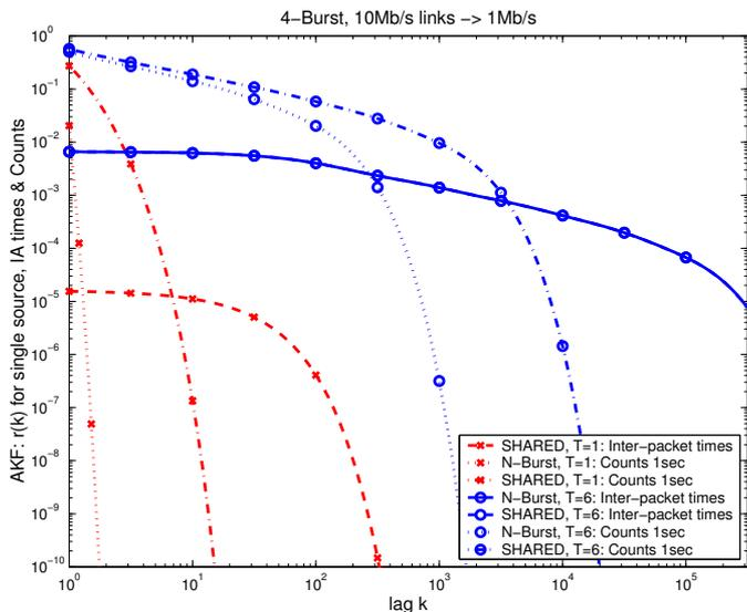
Fig. 3. The autocorrelation function of the inter-packet times and the counting process: The correlation of the inter-packet times of the SHARED model is only marginally larger than in the  $N$ -Burst model when  $T = 6$  (circles). Therefore the two curves are indistinguishable. For  $T = 1$  (crosses), an exponential ON/OFF source in the  $N$ -Burst model shows no correlation in its inter-packet times, that curve does not appear on the logarithmic scale.
