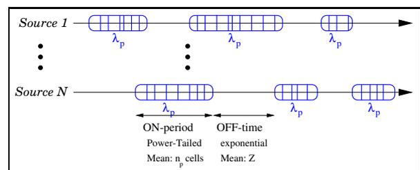
Fig. 1. The  $N$ -Burst Arrival Process: Packets from  $N$  ON/OFF sources are multiplexed together.
