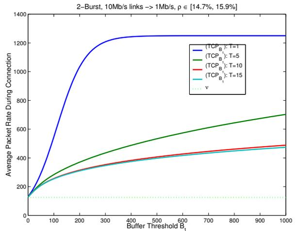
Fig. 6. The average packet-rate during connections of the  $TCP_{B_1}$  model for  $N = 2$  sources: An increased buffer-size  $B_1$  also leads to less throttling. However, the gain is less pronounced for Power-Tailed connection sizes (with large  $T$ ). The uppermost solid curve corresponds to  $T = 1$ , while the lowest solid line corresponds to the highest  $T = 15$  (the same order as indicated in the legend).
