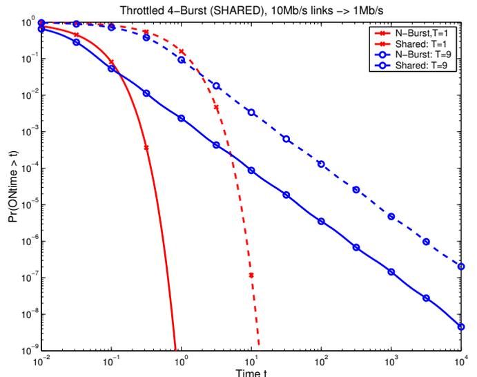
Fig. 2. The complementary distribution function of the duration of the ON periods in the  $N$ -Burst and SHARED model: Power-Tail behavior (appearing as straight line) is observed for both models when  $T = 9$  (i.e. when more phases are used in the truncated Power-Tail distribution, see Appendix B).
