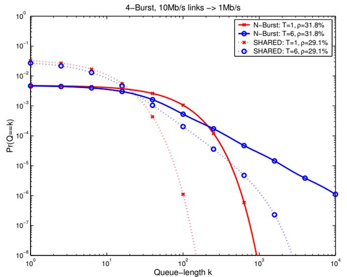
Fig. 4. The queue-length distribution of the  $N$ -Burst and SHARED model: The throttling in the SHARED model (dotted lines) reduces the probabilities of very long queues. This is true for exponential connection sizes (crosses) as well as for truncated Power-Tails (circles).
