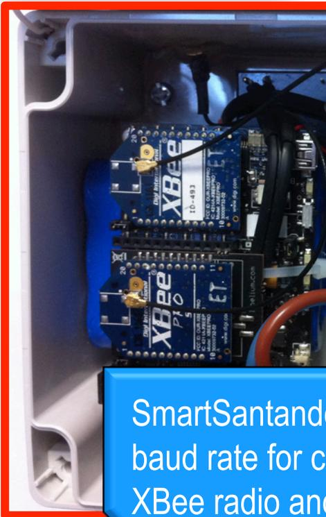
SmartSantander's IoT node uses 38400 baud rate for communication between XBee radio and host ucontroller
