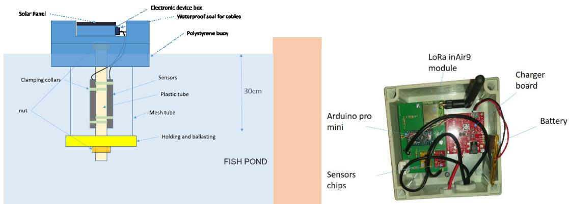
Figure 3: (a) Schema of the first deployed prototype for aquaculture water monitoring in WAZIUP project.
