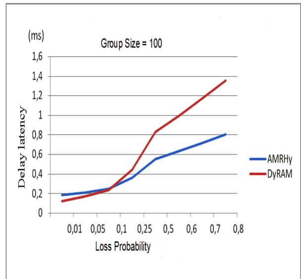
Figure 3: Impact of loss probability on delay latency.
