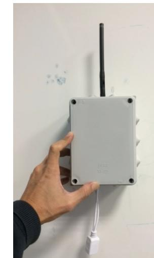
You can have a more integrated version, with a box for outdoor usage and PoE splitter to power the Raspberry with the Ethernet cable. See how we also use a DC-DC converter to get the 5V for the RPI.
