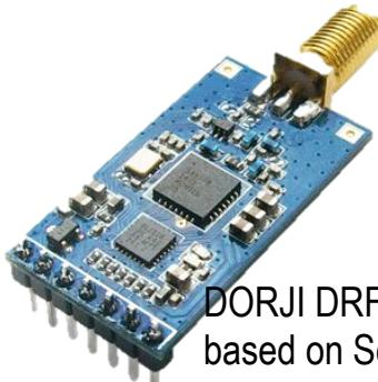
DORJI DRF1278DM is based on Semtech SX1278 LoRa 433MHz
