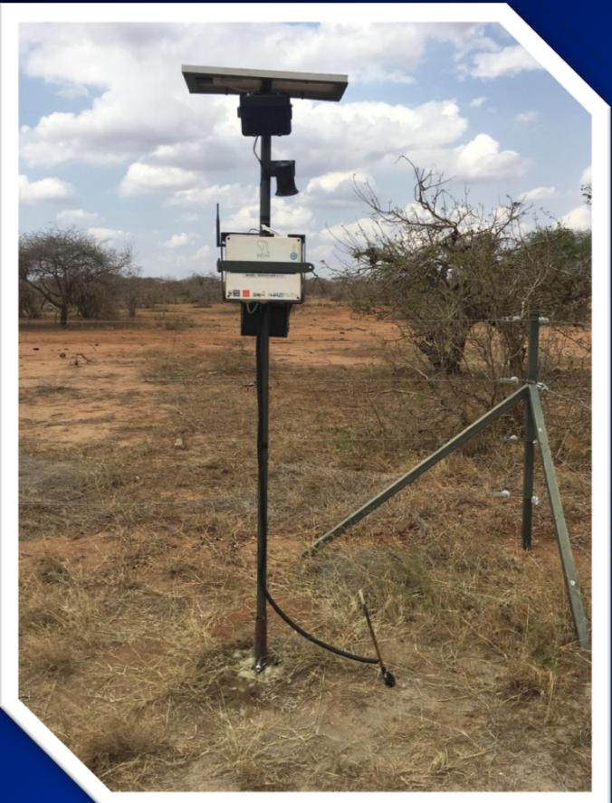
**Detect elephant proximity with infrasonic and seismic sensors**
