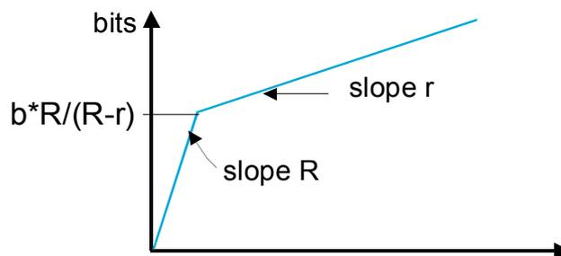
Explain why the second part of the curve above, which indicates the total number of transmitted bits as a function of time, has a slope of  $r$ .
