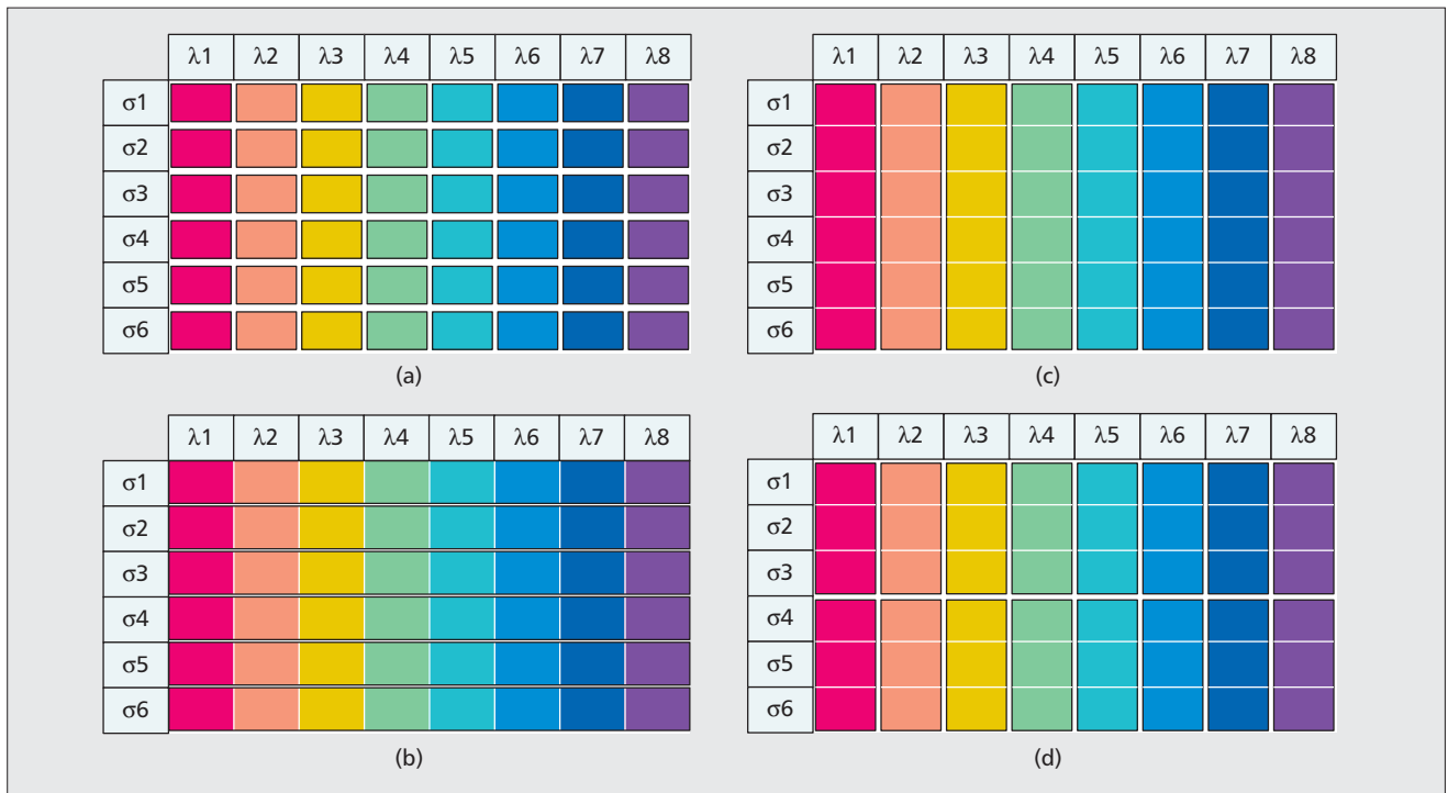
Figure 2. Parsing the fiber’s SDM and WDM channels for switching, where space modes ( \sigma_1, \dots, \sigma_M ) and wavelength channels ( \lambda_1, \dots, \lambda_N ) are fully utilized: a) space-wavelength granularity (each mode/wavelength channel can be independently switched); b) space granularity (switching performed on a mode basis across all wavelengths); c) wavelength granularity (switching performed on a wavelength basis across all modes); d) fractional space-full wavelength granularity (switching performed on a wavelength basis and spatial mode sub-groups).
